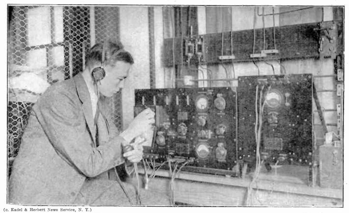
One of the first pictures made of the radio set used for communication with airplanes. It is in operation at the Cornell University Radio School, New York. Very few radio enthusiasts have ever seen a set of this type. A. W. Manahee is photographed at the transmitter.
