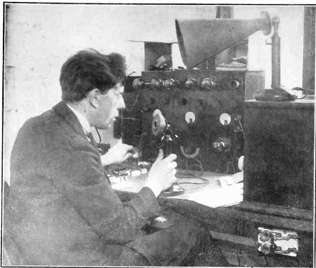
Showing an operator sending music over the wireless phone. The horn is attached to the telephone through which the voice comes. This in turn is sent out through another phone and reaches the receiver. (c. Keystone View Co.)
