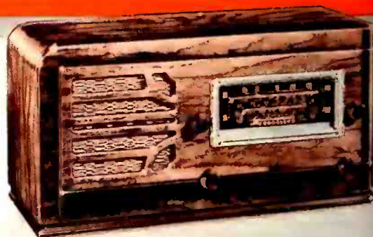
MODEL 24AJ A 7-tube AC with 3 complete bands, 550 to 18,000 Kc. 3-gang condenser, push-pull audio, 8-inch super field speaker, variable tone control, bass compensation. A massive, table-model cabinet, hand-rubbed finish.
