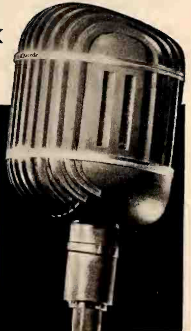
A 639A installation showing minimum feedback. Dotted area indicates dead zone.
