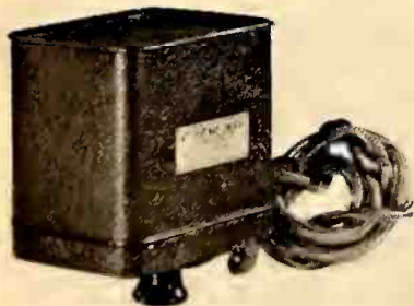
ABC Lab's short-wave police converter tuning 1,600-2,500 KC for use with standard set.
