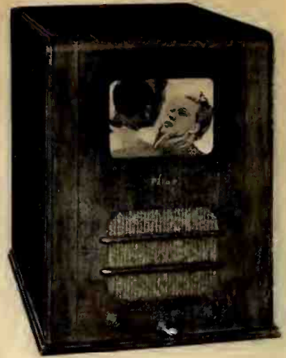
20-tube Pilot model T-90 set using 9-inch tube with black and white picture.
