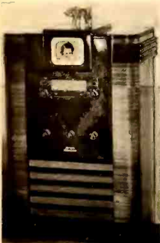
5-inch kinescope featured in this RCA model TRK-5 sight and sound set.
