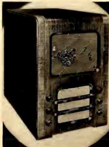
Dumont's table model features a 14-inch tube giving an 8 x 10 inch picture.
