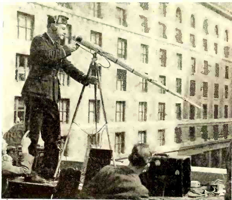
"Machine gun" microphone picks up passing band from nest atop the Empire State Building in New York. WOR engineers used newest Western Electric development.
