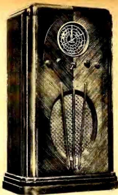
Arvin model 627-B—6-volt farm radio with all-wave tuning and 6 tubes listing at a price of $69.95.
