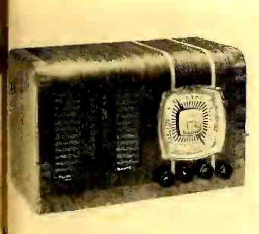
Fada models 351K, 352K, 353K, 361K, 363K—5 and 6 tubes, AC and AC-DC.
