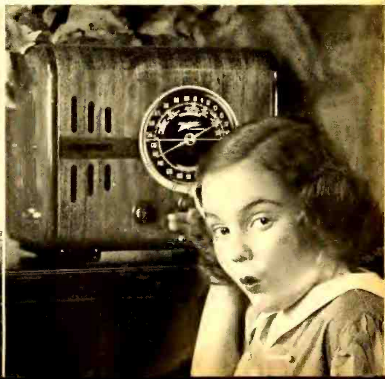
This set works on 6-v. battery, then switches to 110-v. when "high-line" comes.
