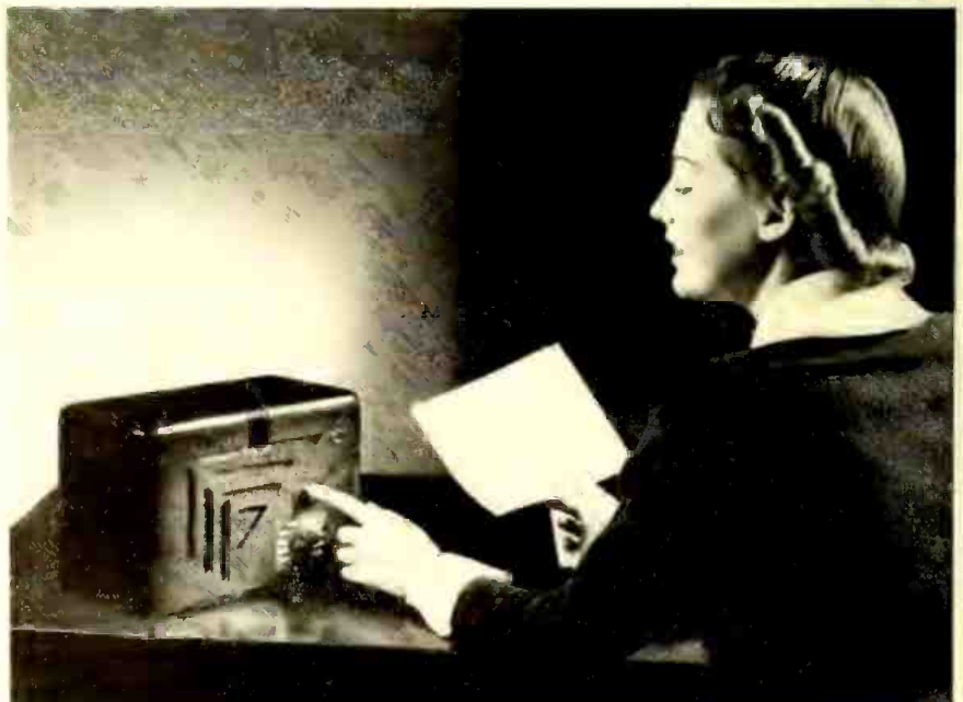
This plug-in office communicating system by Webster Electric, Racine, Wis., provides for selecting any of a number of interconnected stations.
