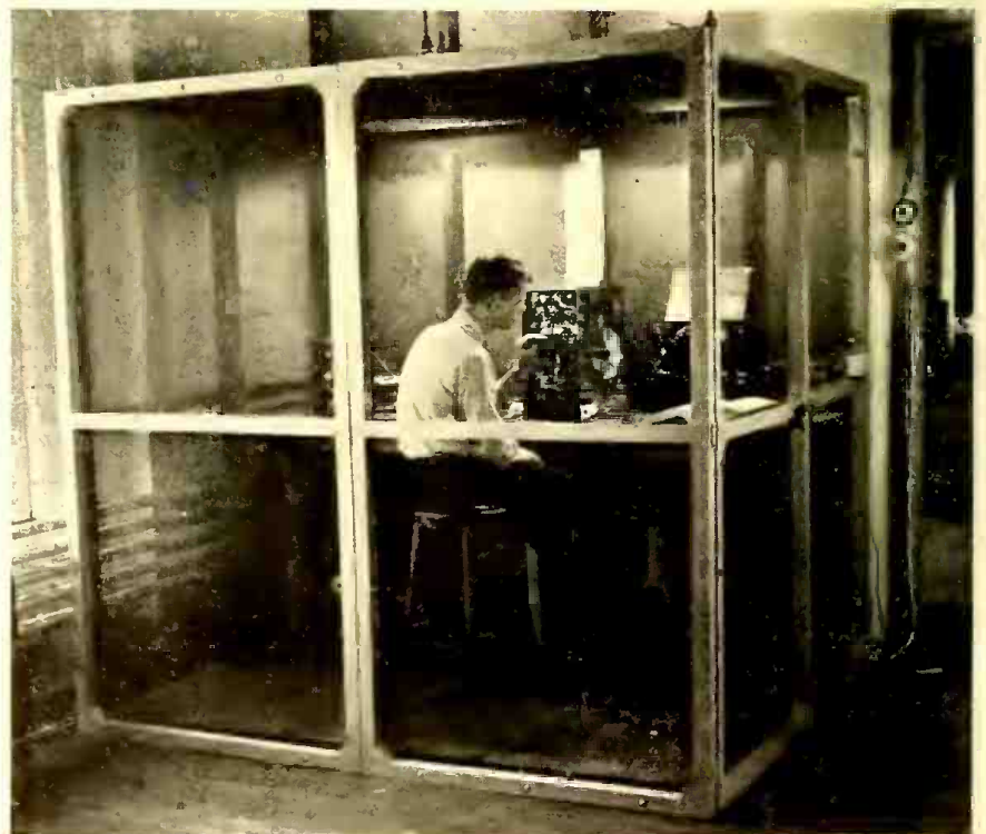
The shielded test room is rapidly becoming one of the "must" items for the service shop. This one is easily constructed, using a wooden frame.
