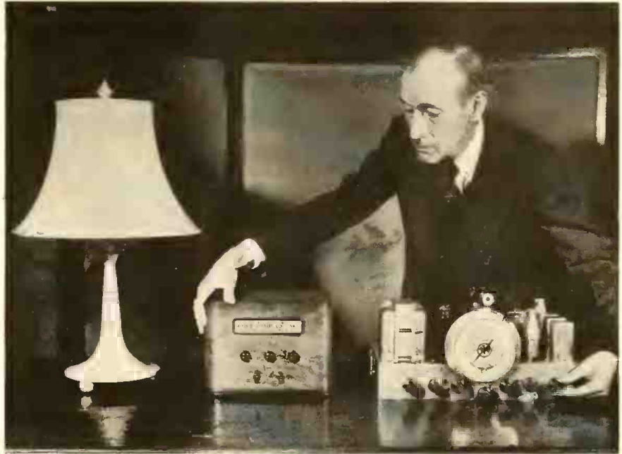
Attractive lamps form the loudspeaker elements of this novel Radio Lamp equipment. The center control box enables sound to be projected through any lamp.
