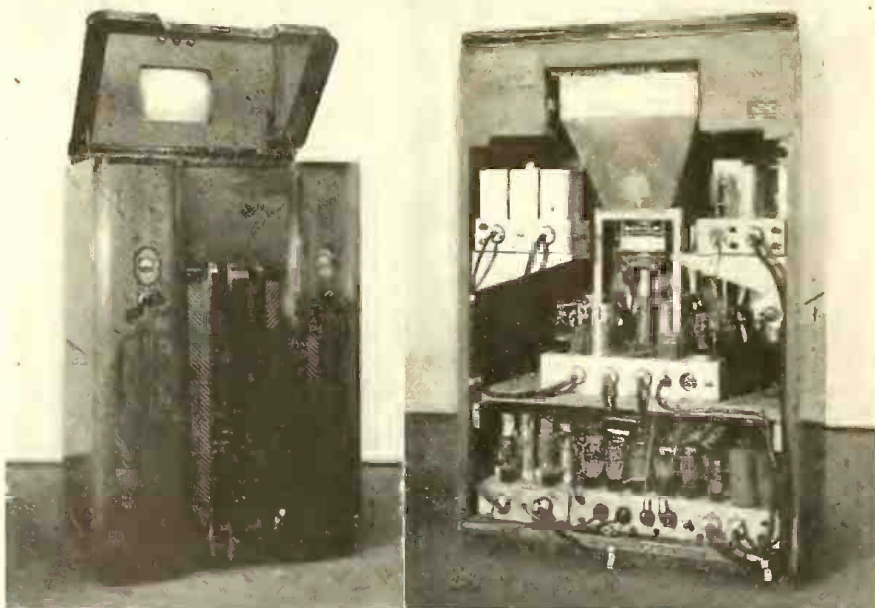
Experimental home-television set by Philco, front and rear. Cathode-ray screen is viewed in 45-deg. mirror. Sound knobs on left, picture-control knobs on viewers' right. Pictures black-and-white, 345 lines, 6-mc channel.
