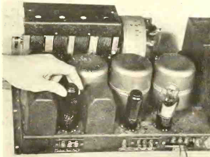
How the new metal-type replacement tubes are installed in an old chassis. An Arcturus Coronet tube being inserted into a "modernizer" or adapter. Center socket shows tube and adapter in place.
