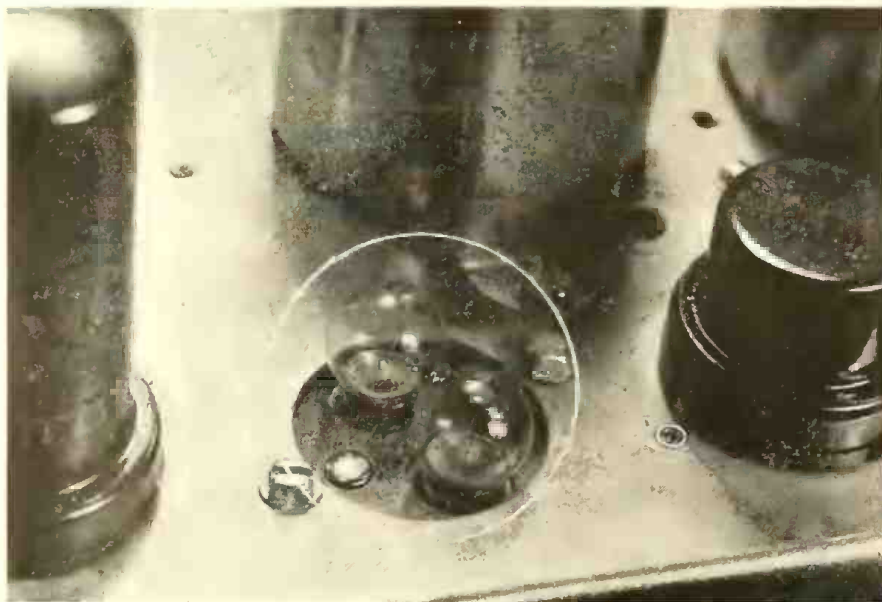
A resistance-variation of volume-range expansion is used in Crosley's "auto expressionator." Maximum-minimum limits are extended, adding brilliance.
