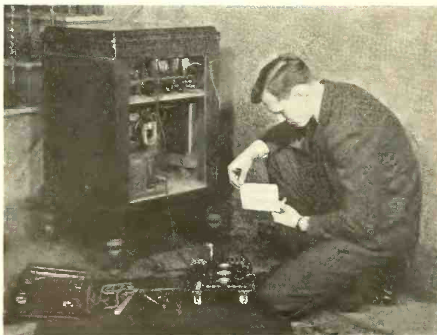
In the home the set analyzer often provides an effective means of determining the general source of trouble. Business-like equipment will foster the idea among radio owners that the serviceman really knows his radios.
