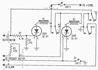
Combination of SCR1 and K1 arms device when ignition is switched on. Triggering stage consists of SCR2 and K2.
