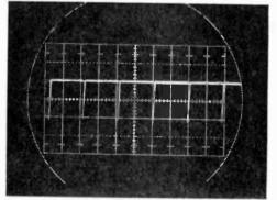
Fig. 5. These rapid timing pulses have amplitude of 2.2 divisions; multiplying this figure by 25 V gives us 55 V peak-to-peak.
