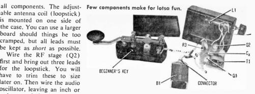
the metal collar snaps snugly in place when the coil is pushed in. Make sure that the perf board, loopstick, and battery fit easily into the case. Connections should be as rugged as possible.
