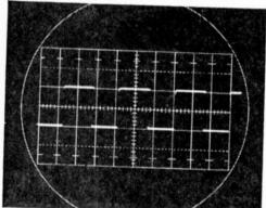
Fig. 1. Square wave serves as calibrated voltage source for accurate scope displays.
