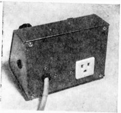
Front and rear views of completed Autodim. Unit is plugged into AC outlet; slide projector plugs into socket at rear of Autodim. Because of this arrangement, switch S1 must be on for projector to operate. Note position of grounded, three-prong socket (J1) at rear of unit.
