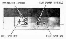
Straightforward as an amplifier can be, Stereo 120 is clean and uncrowded as they come. Business-end of amplifier has only input jacks and speaker terminals; line cord and power switch are on opposite side.
