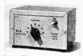
Booster covers entire BCB with single tuning capacitor. No calibration is necessary—you simply tune for maximum signal.
