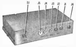
Insulated jacks J1 through J6 provide separate output for divider network. Pin jacks were used, but you can use other types.
