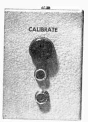
RF jacks on rear apron mate with existing transmission line connectors. Calibration control, once set, needn't be reset if power remains same.
