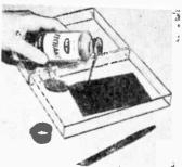
To use 500 kit, you trace outline of PC foil layout on board, trace around outline with resist pen, then fill in larger areas with resist. Etchant takes approximately 20 minutes to do its job.
