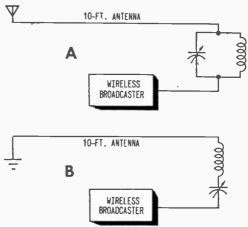
For one thing, at the fade-out point you have a parallel, resonant wave trap in series with the antenna. The wave trap blocks passage of your signal.
