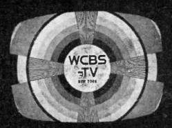
Typica TV test pattern is transmitted perfectly round, perfectly centered, and with all wedges of equal length. Height and width have 3:4 ratio.
