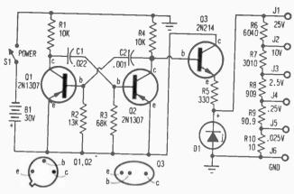
Multivibrator (flip-flop) circuit produces square-wave output at frequency of 1200 Hz. Buffer stage (Q3) prevents loading of oscillator by zener diode (D1) or external circuit.
