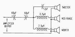
Here's a diagram of a crossover network for 8-ohm speakers. If you use 16-ohm speakers, the capacitors should be half the listed value. As to exact frequency crossover, juggle the values of your capacitors and chokes until you get what sounds best to you.
