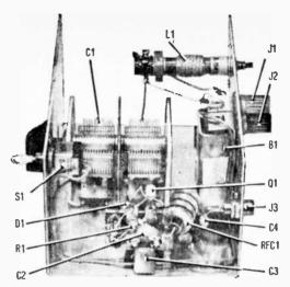
Author used miniature power switch for \$1, but any spst toggle switch will work. Locate RFC1 as far as possible from coil L1.
