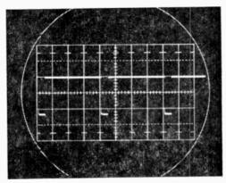
Fig. 2. An unsymmetrical waveshape can be corrected by adjusting the value of R2.
