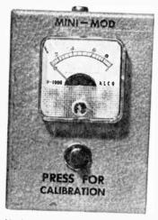
High-speed meter has expanded scale between 0.2 and 0.8 so CB accessories such as speech compressors and clippers can be readily adjusted.
