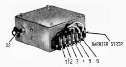
Barrier strip provides connections for car's electrical system. Type of trigger switch and alarm mechanism you use are up to you.
