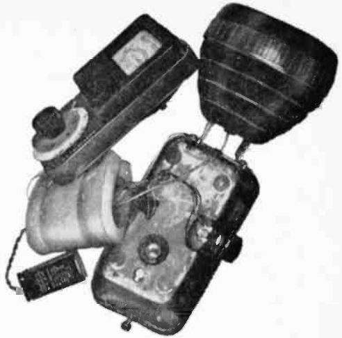
Completed unit shows circuit board wrapped in foam and secured with transparent tape.
