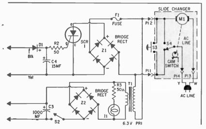
Large shaded areas show original circuitry of prewired units used in Tape-Slide Synchronizer. Added circuitry is outside of shaded boxes.
