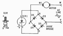
Unique basic circuit is heart of Slide Synchronizer. Power-line AC flows through motor M1 but DC flows through SCR1 by way of diode bridge—simple and inexpensive.
