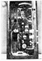
Slide-rule dial in radio author used was permanently affixed to plastic cabinet, so author carefully sawed it out with hacksaw blade. Dial could then be fitted into cutout in telephone box.
