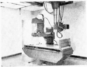
Modern X-ray installation (at left) conceals X-ray tube in rayproof body of enclosed table, while image is now made thousands of times brighter by means of image intensifier on deck extending across table. Further, over-table X-ray tube is supported on telescoping column, in turn suspended from overhead carriage traveling on ceiling racks. Resulting arrangement permits rapid positioning and angulation of X-ray tube.
