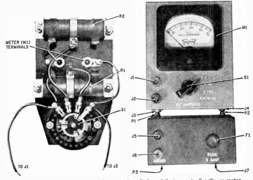
All circuitry inside meter case (left) is on phenolic board that mounts directly on meter terminals. Tapered end of phenolic board is to give better clearance for leads to J1 and J2. If you start with a larger case, adapter can be built in, eliminating J3, J4, J5 and J6 as well as P1 and P2. The 5-amp fuse will not protect M1 if shunt resistor should open up.
