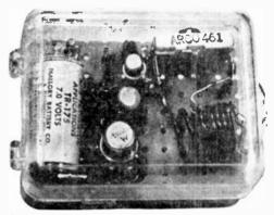
Tight-wound portion of L1 is a loading coil for the short antenna—the spread portion tunes with C5. Leads that connect to the base, emitter and collector of Q2 should be kept as short as possible (a normal VHF wiring technique). Those to Q1 aren't as critical. Transparent plastic box protects delicate parts—specially L1 and C5—from damage.
