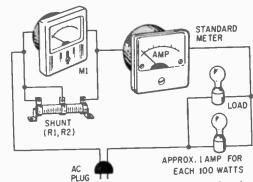
You don't need to resort to a lot of figuring if you use the cut-and-try method of shunt design. Just connect the two meters in series and increase the resistance of the shunt until meters indicate the scme. Refer to the text.
