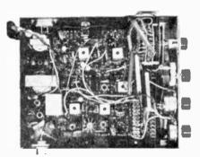
Since output jack is part of printed-circuit assembly, entire transceiver can be removed as unit for service and adjustment.
