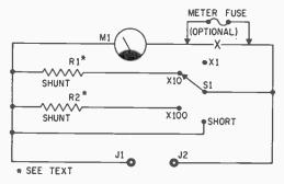
ance figures out to less than one ohm it may be necessary to make it from copper or nichrome wire. Remember it will be necessary to multiply the scale readings by 100 when using this shunt. You can use the same formula to figure other values of shunts.
