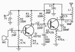
Circuit is simple but you must remember that wiring at 100 MHz is critical—all leads to Q2 and L1-C5 must be kept short to get proper operation on the FM band.
