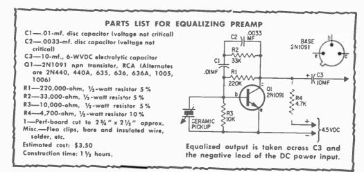
Layout of the components on the perforated circuit board is not at all critical—but watch ground connections if you take power from amplifier.
