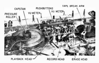
Top view of unit shows location of heads, VU meters, and pushbutton controls. Use of pushon terminals on leads to and from head and between transport and printed-circuit board obviates need for soldering.
