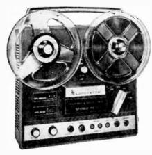
reset button, stereo tape head output jacks, 2 inputs for mike and auxiliary. Response is 40-15,000 Hz at 7½ ips; 40-10,000 Hz at 3¾ ips. Signal-tonoise ratio is 40 db or better; crosstalk 55 db or better. Size is 11% x 1¼ x 6¾ inches. Takes 3-to 7-inch reels. Comes with dynamic microphone, 3 connecting cables, 2 rubber reel caps and 7-inch empty take-up reel. Textured vinyl case. Model RK-810 from Lafayette Radio Electronics Corp., 111 Jericho Turnpike, Syosset, N.Y. 11791.
