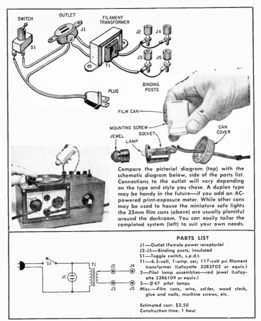
The lamps are powered by a 6.3-volt filament transformer which is enclosed in a small wooden box at one end of a board used for a base—the front portion of the base supports the timer itself. The various dimensions of the box are adjusted to suit the size of the timer. The top of the box holds a line switch and four binding posts; the right side, a single AC outlet—for the timer's AC plug.
