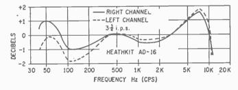
Fig. 1. Record-play response of Heath AD-16 at 3 3/4 ips was in keeping with company's claim of ± 3 db, 30 to 10,000 Hz. Note that both channels offer approximately the same response.
