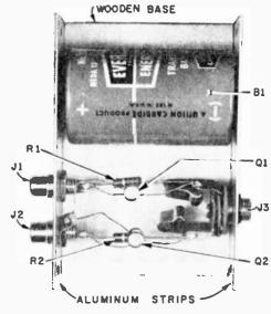
Aluminum panels attached to wooden base form sides of unit and also serve as battery holder. Jacks need not be insulated.
