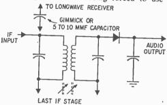
The 5- to 10-mmf capacitor reduces detuning of IF amplifier to a minimum but after the connection is made last stage should be repeaked. IF signal goes to longwave receiver through a short length of coaxial lead.
