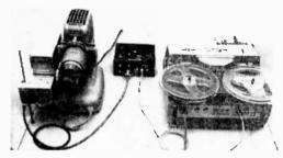
Complete setup, ready for an automated slide show, has Tape-Slide Synchronizer between slide projector and tape machine. Use any automatic projector, stereo unit.
