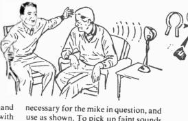
necessary for the mike in question, and use as shown. To pick up faint sounds attach the lamp's bowl-type reflector to the lamp's socket to "funnel" or focus the sound into the mike. Face the mike toward the inside of the reflector. Position mike closer or further from the bowl for best pickup.
