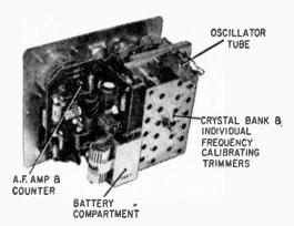
Operating panel of the International Crystal C-12B (left) and internal layout (above) shows the major portions of this accurate (±100 Hz) frequency meter for CB.
