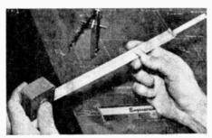
B and C scales provide an endless feature formerly found on circular slide rules. Reverse side measures to 20 in. or its metric equivalent and lists basic equivalents, fan laws, power, trig and geometric formulas. Cost, \$8.50; manufacturer, CalTape, 1095 Kingston Park, Roann, Ind. 46974.
