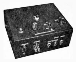
This vertion of Tape-Slide Synchronizer has top-of-the-cabinet lettering facing operator. Cables come out of unit on the side of cabinet away from the operator.
