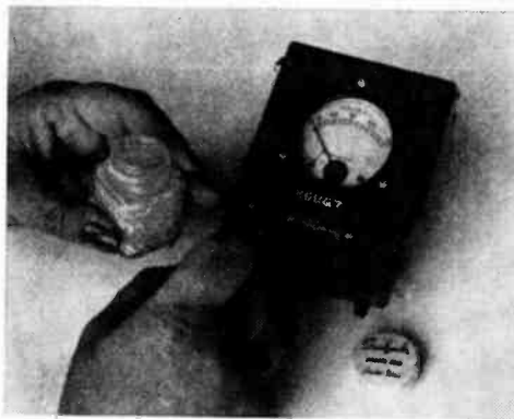
White ink, such as the type used in photo albums, is suitable for labelling dark colored equipment—cheapest and quickest method.
