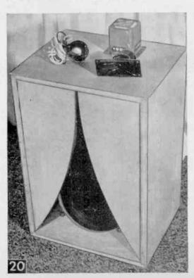
Medium and low-range speakers come with this enclosure. Tweeter, control and crossover on top will be mounted in cabinet outside this enclosure.
