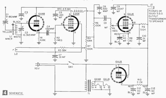
This receiver's tuning range, from 85 to 550 Kc, is covered in two adjustments of the core on L1. When set to receive 550 Kc at C2's minimum capacity, the receiver will tune down to about 200 Kc. The range from 85 to 200 Kc is tuned when the slug is almost fully inserted into L1. Overlap on both bands will
