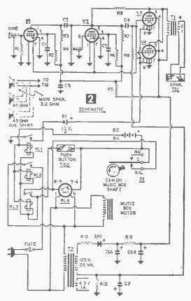
cause it would be sensitive to the hum resulting from the magnetic field that surrounds the motor. A vibration pickup mike, as used for electric guitars and similar musical instruments is also impractical, because of its sensitivity to the mechanical noises generated as the motor and its associated gearing operates.
