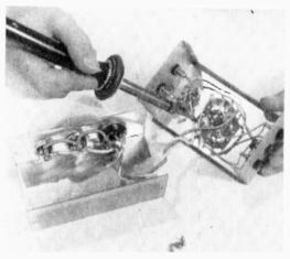
Fig. 2: Tube filament checking sockets are optional. Wire your chassis connections with solid hookup wire, and use flexible wire for the tube socket connections.
