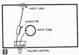
Leads likely to pick up hum. Remedy is to substitute shielded cable, dressed close to chassis.
