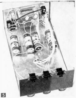
Studio unit is easy to wire. Arrow shows rectifiers mounted on aluminum heat sink bracket. Capacitor polarity is important and must be correct. For heavy duty use, add a small fan and ventilating holes.
