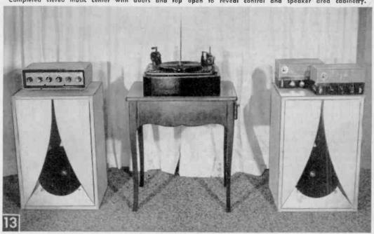
Without cabinet, the equipment looks like this: preamp over one speaker enclosure, amplifiers (to be remotely installed as in Fig. 2) over the other, record player. Tuner and tweeters not shown.
