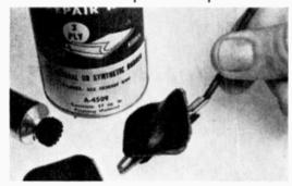
• When small, bare uninsulated test clips are used on 'hot' wires connected to live circuits, insulate the clips with rubber-tire patching. When ordinary clip insulators aren't available, tire-patching covers come in mighty handy. Simply sandwich the clip between two of the patches and bring the outer edges together and squeeze. The adhesive on the patching is sufficient so you won't need to use rubber cement.—J. A. C.
