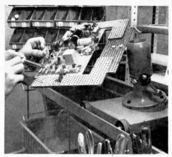
Power arm mounted on a dolly conveyor lets you angle and position work for convenience. You cover track with a formica top when not in use. "Swiss cheese" fixture that holds circuit board here costs about \$19.
