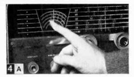
Here's how you can easily tell if a set has general coverage, will pick up all the bands shown in Fig. 3. In 4A, finger points to 4.5 megacycles, which is at extreme left of the second band on the dial. In 4B, finger points to 4.6 megacycles, which is on extreme right of the third band; thus there is no gap between the bands. In 4C, though, note that the top band runs from 3.5 to 4.0, while the band below it picks up at 7.0. This receiver covers only the ham bands.
