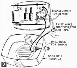
transformer from its terminal and connect one of the pigtail wires on the switch to the transformer terminal. Then connect the transformer wire to the other pigtail wire on the switch by twisting them together and taping.
