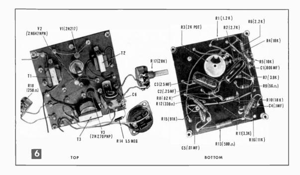
tortion. Transistor V2 amplifies the signal and isolates the oscillator from the output stage. This isolation improves oscillator stability since it prevents any change in the bridge circuit from reflecting back to the oscillator.
