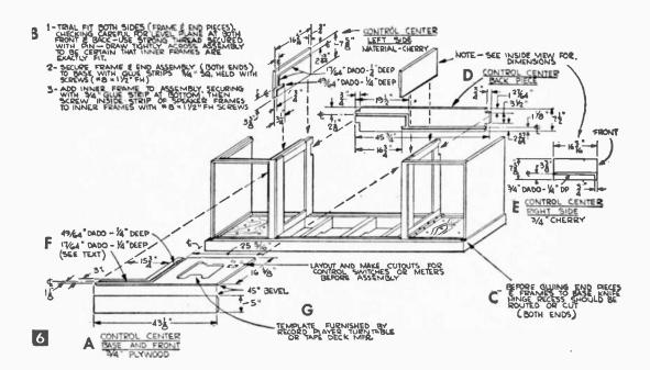
Cut two  $16^{11}/_{16} \times 18^{1}/_{8}$ -in. pieces from the  $^{3}/_{4}$ -in. plywood sheet for end panels, then dado and notch as in Fig. 7D. Cut and dado the solid cherry front and rear top pieces and the birch plywood back as in Fig. 7E.
