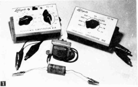
These basic passive components plus a 6.3-volt transformer and an ac voltmeter are all that's needed for some challenging ac experiments.
