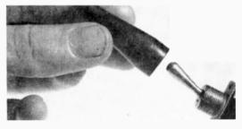
To avoid any possible shock from the bathandles of toggle switches, place plastic test-clip insulators over them. These insulators are also good dust covers to prevent particles of metal and other foreign materials from entering the switch mechanism.
