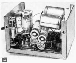
Inside the portable case, arrow shows power rectifiers mounted in battery clip used as heat sink. Capacitors are taped in place after assembly.
