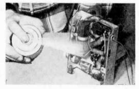
haves or goes dead. The trouble may be a part that expands with heat after current has been flowing through for a few moments. Spray suspicious parts with CO, gas one at a time. The intense cold will contract a defective component so it can work normally.
