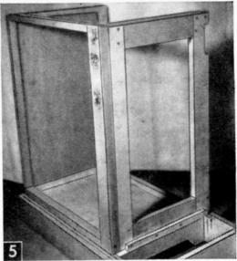
Lap-jointed inner frame is supported by heavy member of sub-base. Pine components are concealed by solid and veneer cherry in finished cabinet.
