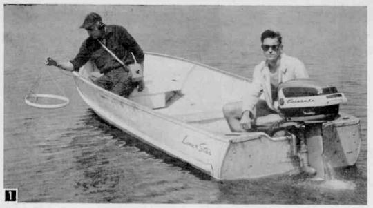
S&M Boat Designer Bill Jackson demonstrates search method. A 26-in. loop is wired into a 100-ft. cable made of lamp cord. When the coil approaches the metal object, a change in tone is heard.
