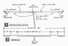
IMITED in antenna space? Here is an inexpensive three-band system that will fit the average backyard and is ideal for the novice amateur operator since it's designed for 80, 40, and 15 meters.
