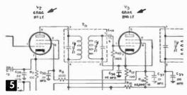
It's easy to tell how many i.f. stages a communications receiver has. Just take a close look at its schematic diagram. The stages (arrows) will be clearly labeled as shown in this section of a typical schematic. This set has two i.f. stages.
