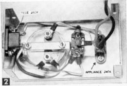
Interior view of tester showing parts placement.
