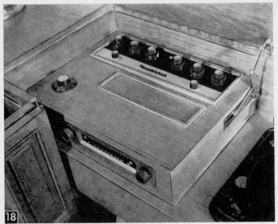
Tuner-preamp case in place. Note ventilator panel and single dial at left which controls tweeter mounted in top outside corner of speaker cabinet adjoining. Tension of bracket can be set to hold lid open as desired.
