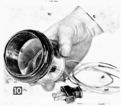
Small coil locates nails and tacks in walls and tires. A  $\frac{1}{4}$  brad can be detected at 2 inches.
