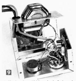
Inside view shows Mini-Amp chassis. Device to be tested plugs directly into receptacle on top. Power line (arrow) feeds through opening in transformer. Transformer secondary winding output is amplified and feeds to test leads. R3 is common terminal.
