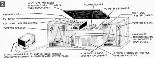
Minimum acceptable distance for placement of speakers is 6 ft., which provides a stereo zone 11 to 17 ft. from front of cabinet. Low- and mid-range speakers are spaced on 6-ft, centers. Tweeters are placed further out to extend the stereo listening area.
