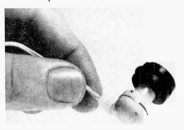
• To reduce the volume of an earphone of the "earplug" type when using the phone in conjunction with a set that has insufficient volume reduction at its lowest setting (this happens often near stations) slip a soft rubber grommet over the phone. This keeps it from fitting into your ear so far, yet still allows it to fit firmly. The lengthened distance between phone diaphragm and ear drum lowers the volume several db's.—John A. Comstock.
