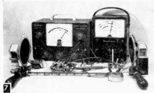
Set-up for voltmeter method of finding speed of sound.
