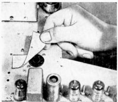
• When soldering on top side of radio or TV chassis, dropping solder in an open tube socket can cause trouble. Eliminate this possibility by placing a strip of wide adhesive tape over the open socket.—H. LEEPER.
