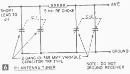
terference can be minimized by reducing the antenna coupling or, in severe cases, by the use of the simple Pi antenna tuner (shown in Fig. 6). The tuner can be built on a small pine block. Adjust C1 and C2 for minimum BCB interference.
