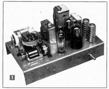
With this device hooked into your front door-bell circuit, you substitute the soft, tinkling tones of a music box for the jangle of bell, rasp of buzzer or raucous cling-clang of chimes
