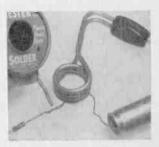
the heater coil turns and plug the heater in intermittently until the joint gets hot enough. Use the heater to aid heating large work when your iron or gun isn't large enough to handle the job.—John A. Comstock.
