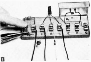
Front view shows breadboard set up as crystal detector with one stage of audio. Rear view shows power transistor bolted directly to copper heat sink mount. Engrave the symbols with a ball point pen.
