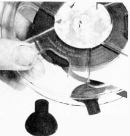
Need a good pair of recording tape spool locks for your tape recorder? A pair that isn't easily misplaced when not in use? Two medium-size rubber suction cups—the type with open tops—are ideal for this purpose. The cups are easy to slip over the spindles to hold the spools, or they may be used as wedges to hold tape on the spools. When they aren't in use, you can store them neatly on the tape deck by means of suction. They might be used this way as holders for your regular spool locks.-J. A. C.
