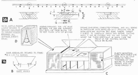
Opening dimensions depend on style and make of units to be installed. Most preamps can be installed in any position but some tuners cannot. Check units before cutting wood. You may, if possible, choose to mount the tuner vertically, in which case the control section would be blank.
