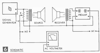
Schematic for determining velocity of sound with an ac voltmeter.
