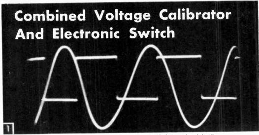
Sine and square wave seen simultaneously with aid of electronic switch unit.
