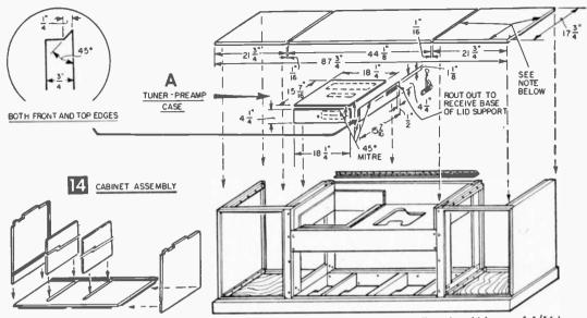
Note: Dimensions given for top panels are finished measurements. Be sure to allow for thickness of 1/16-in.
