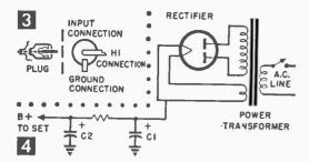
A broken shield or disconnection from plug ground or a faulty or open input jack can cause hum pickup.
