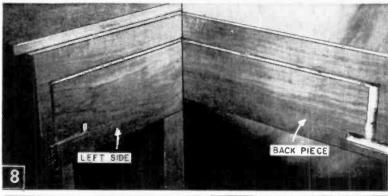
Views of left and right sides of control center back piece, after fitting side pieces. Note perfect match of dadoes at each end. Right side piece is cut about 1 in. narrower than recommended in Fig. 6E.
