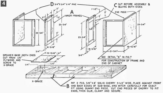
Caution: Assemble subframe before gluing. After checking for squareness, cut X-braces for each end. Disassemble, glue, and complete assembly, including braces. Check for perfect squareness.
