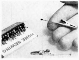
• Perhaps the easiest way to color-code test clips used for marking circuit wires or parts to aid servicing is to attach a colored dressmaker s pin to each clip. The colored head of the pin sticks out like a sore thumb against wiring. What's more the pins are inexpensive and available in dozens of colors.—J. A. C.
