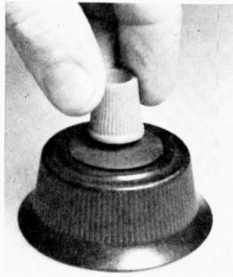
When the turning ratio of a large knob on a receiver is too slow, a rubber suction cup will solve the problem. Place the cup directly in the center of the knob and use it as an additional knob for fast tuning. A bottle-cap force-fitted into the cup (or over the cup) will make turning easier and improve appearance.-J. A. C.
