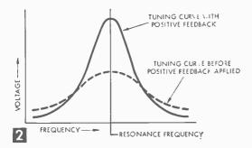
$$\begin{array}{l} \text{Gain with} \\ \text{Positive Feedback} = \frac{\text{Normal gain}}{1 - \text{Normal gain}} \\ \times \text{Feedback Ratio} \end{array}$$
