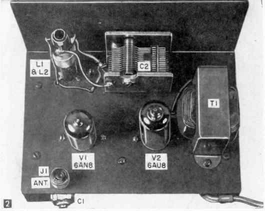
Topside of the receiver's Masonite chassis. The antenna coil, L1, is mounted so that its slug is adjusted from below the chassis.
