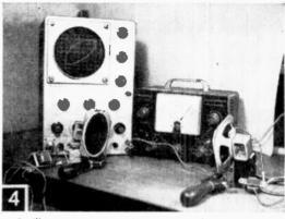
Oscilloscope set-up for determining velocity of sound.
