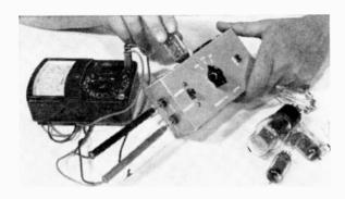
Fig. 6: Tube checking circuits on side of box are handy extra feature for radio and TV servicemen working on sets in homes. Binding posts for other kinds of tests can be added to this handsome case.
