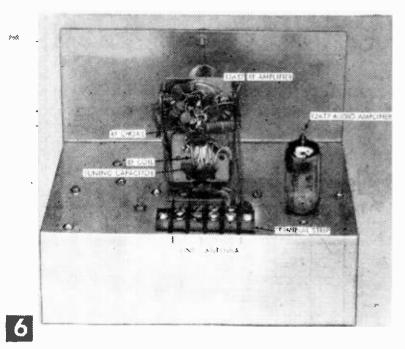
The RF detector unit is in the center in this top-chassis view. This unit is wired in late in construction.
