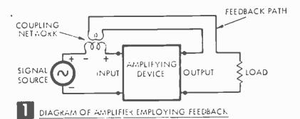
NE of the truly valuable techniques available to the small-receiver designer is positive feedback, or regeneration. Most small receiver projects utilize it; in fact, all truly sensitive receivers using less than five tubes or transistors probably apply this principle.
