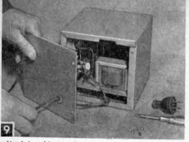
Notch in cabinet to clear transformer will be covered when side panel is attached. Note knot in line cord to prevent any unintentional strain from loosening input connections.
