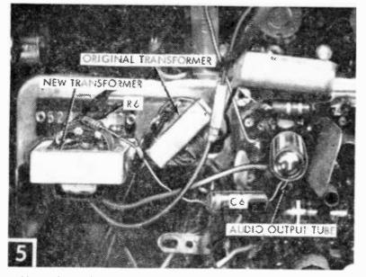
Mounting details of the substitution of a higher impedance output transformer to match the 16-ohm impedance of the hi-fi speakers.
