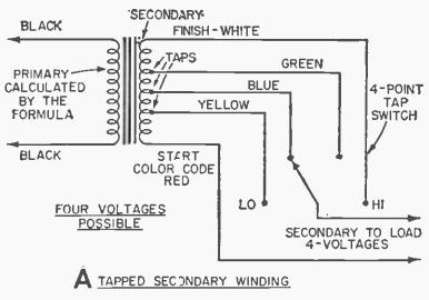
FIGURE EACH TAP FOR A SINGLE VOLTAGE TURNS = DESIRED VOLTS X TURNS PER VOLT RATIO - 6 % FOR LOSSES. (SEE TEXT)
