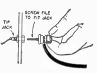
ing a binding post with non-removable tops and molded-in screw-shanks (such as made by Eby), simply file the screw-shank to the same diameter as a phone cord tip.—A. TRAUFFER.
