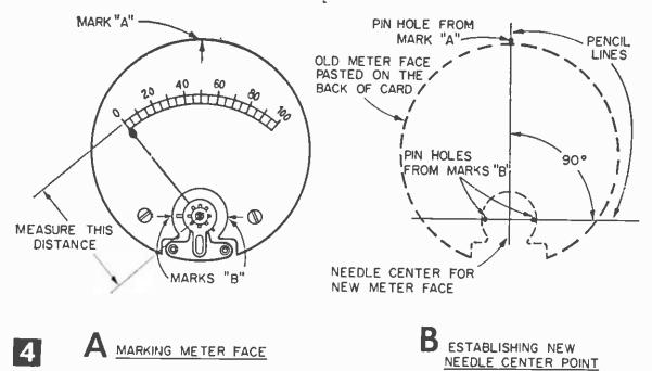
How the radius and length of the meter scale can be transferred to the card stock pasted on the back of the dial plate.
