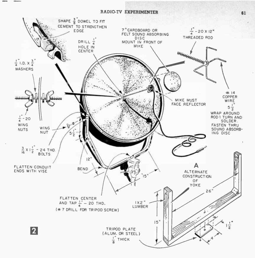
handles, and locate the center of the 26-in. dish by laying a yardstick across at the widest point and drawing a line. Then lay the yardstick across again, at a right angle to the first line and mark an X at the disc's center. Drill a ¼-in. hole for the threaded microphone support rod.
