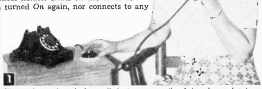
Silencer button by telephone eliminates conversation being drowned out by radio or TV set.
