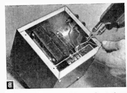
After chassis is placed in cabinet, panel connections are easy to complete through side openings.
