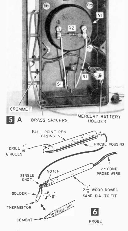
After the joint is cool, with a needle or small probe gently bend the other thermistor lead until it lays parallel to the first one. Solder as before. Then carefully ease the bead end of the thermistor into a point about <sup>1</sup>/<sub>8</sub>-in. across, so it projects straight forward from the section of wire feeding into the wood dowel.
