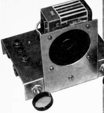
Here's a complete sound system that operates without a-c power. A built-in preamp permits use of dynamic mikes, reluctance type pickups as well as crystal phono pickups.
