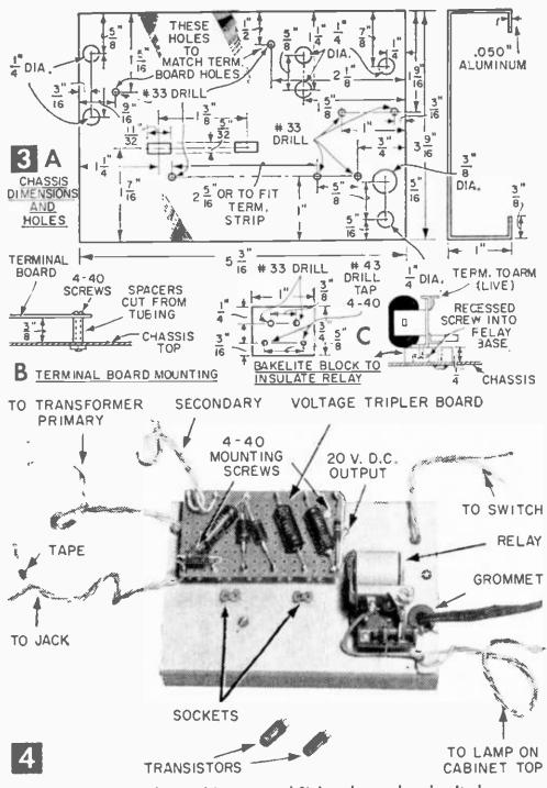
Compact terminal board is mounted ¾-in. above chassis. It changes a-c to d-c and triples the transformer voltage to do the work of a battery constantly and without need for frequent replacement.
