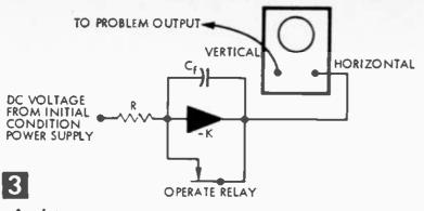
An integrator can generate sweep voltage for CRO display.
