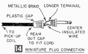
in., then solder insulated center wire to short terminal connected to end of plug. Solder metallic braid to the longer terminal, which is grounded. Snip off any stray ends to prevent touching the wrong terminal and screw cap in place over connections.
