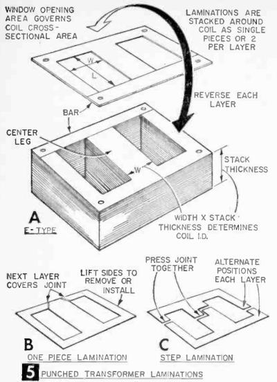
STACKED LAMINATIONS ARE "26-"29 GAGE, SILICON TRANS-FORMER STEEL. FOR 60-400 CYCLES, USE #29 GAGE TO LOWER LOSSES. ("29 MAY BE USED ON LOWER FREQUENCIES)
