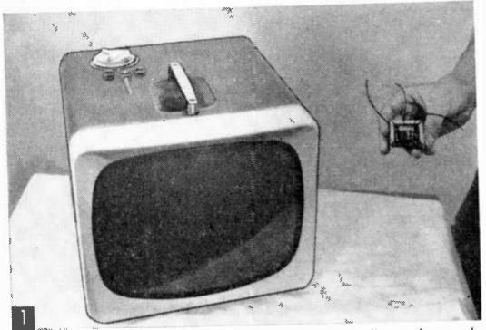
The CR tube brightener usually cures dimness, when the dimness is caused by low cathode emission.
