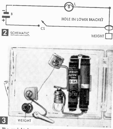
The weight is suspended on the bare wire, which passes through the hole in the lower bracket. If wire touches bracket, bulb lights.
