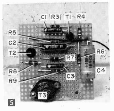
Amplifier parts are mounted on Bakelite piece.
