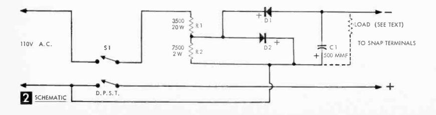
House-current is converted by this unit to power transistor radios. If battery is left in radio, unit will charge it while powering the radio.
