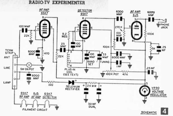
When the VR tube lights up properly, remove the line-cord plug and insert the rest of the tubes in their sockets. Connect a 40-watt lamp bulb (any other size bulb may damage tubes) to the terminals marked "lamp" in Fig. 4. Plug into the line again and turn on the line switch. If the filament circuit is satisfactory, the 40-watt lamp bulb should light up to nearly full brilliancy. Removing any tube except the voltage regulator will cause the lamp to go out.
