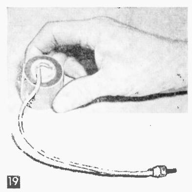
Microphone mounted in insulating rubber ring, which in turn is fitted into Bakelite tubing mouthpiece.
