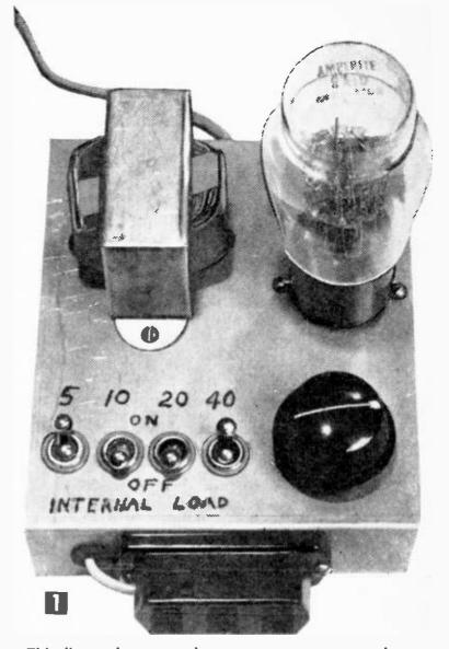
This line voltage regulator assures constant voltage for experiments.
