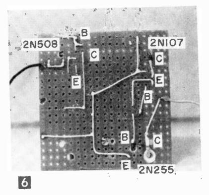
Underside view of amplifier chassis shows wiring.
