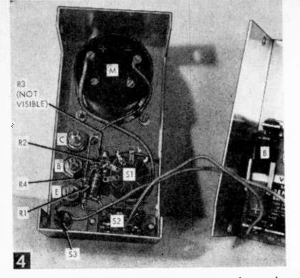
This inside panel view shows parts mounting and wiring.
