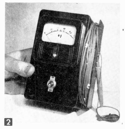
Fig 1. Lower the probe into the water, flip the switch, and the meter instantly reads the temperature. Fig. 2. The meter scale is labeled to read directly in degrees F. Left-handed fishermen will want to mount the wire reel on the opposite side.
