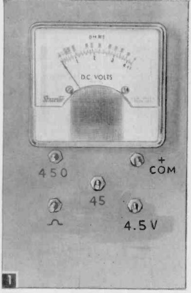
This inexpensive volt-ohmmeter employs machine screws as terminals for Mini-Gator clips on test leads.
