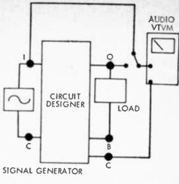
INPUT - OUTPUT CIRCUIT INSTRUMENTATION FOR HIGH GAIN AMPLIFIER DESIGN AND FREQUENCY RESPONSE MEASUREMENTS
