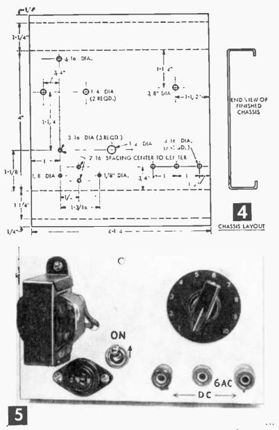
Top view of the low voltage power supply.
