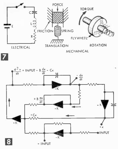
ratios of input and feedback resistors and capacitors in the hook-up. The computer hook-up for solving this differential equation is shown in Fig. 8. The initial conditions are assumed to be zero at the beginning of the problem in this case, and A equals 1.
