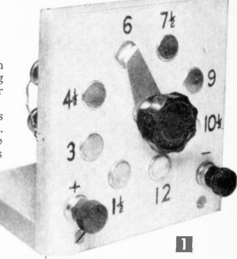
Bottoms of small flashlight cells act as rotary switchpoints in simplified power supply designed especially for transistor experimenters.
