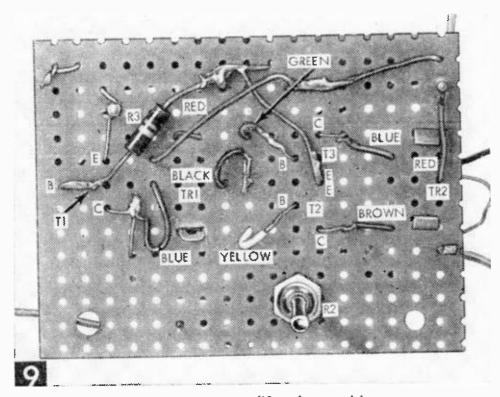
Bottom view of amplifier shows wiring.
