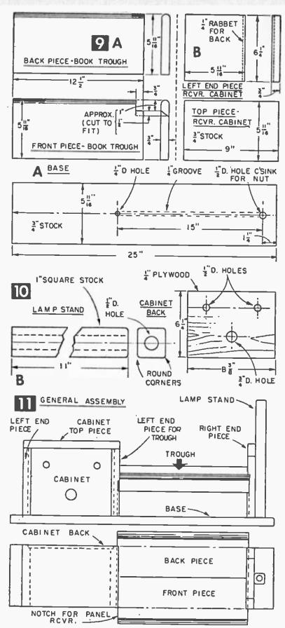
nect about 3 ft. of rubber-covered lamp cord to the socket and assemble after passing the cord down through the lamp tubing to the bottom of the base. Run the lamp cord through the groove and pass it up through the ¼-in. hole into the cabinet.
