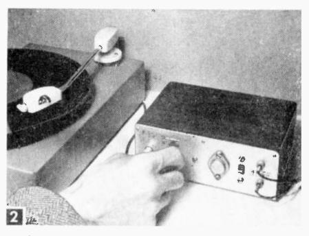
With a crystal pickup and an extended range 8 or 12-in. speaker, reproduction is crisp and clear with volume to fill a room.
