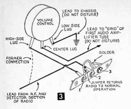
Radio Now Works as Phono Amp. Connect the leads of a crystal or ceramic phono pickup to the Audio and Ground terminals (Fig. 4); if your radio has a good a-f section and a respectable speaker, you'll get quality music. If your amp section is low gain, use a high output crystal, or ceramic phono cartridge. Otherwise, if your amp section has plenty of gain, you can use the higher quality low voltage crystals, or ceramic cartridges as are made by Ronette, Electro-Voice and Sonotone.
