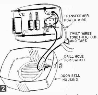
transformer from its terminal and connect one of the pigtail wires on the switch to the transformer terminal. Then connect the transformer wire to the other pigtail wire on the switch by twisting them together and taping.
