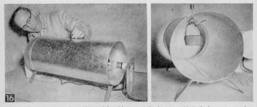
Use a 10-inch stovepipe and two 250-watt infrared lamps to make the oven. With the knob you can turn the coil during baking.
