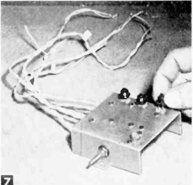
Test-mounting three audio transistors in their sockets. Leads from these transistors will need to be cut off to about 7/16-in. length with diagonal pliers, but transistors should not be permanently placed in sockets until megaphone assembly is complete, ready for cover plate to be put on (Fig. 2A). Wire leads to batteries, switch and speaker are identified with marked tabs of white tape to assure correct connections. Plus battery lead is also marked to avoid error.
