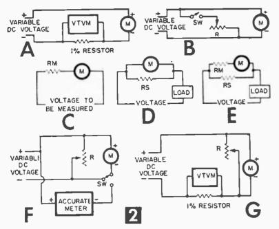
Schematics (A) for determining the basic meter movement, if unknown, (B) for determining internal resistance of a meter, (C) for determining a meter's voltage rating, (D) showing connection of meter shunt, (E) showing how to increase meter voltage rating by using a multiplier and current shunt, and (F and G) circuits for determining the amount of resistance wire to use in making meter shunts.
