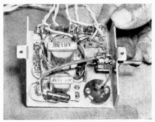
Underside of amplifier chassis, with parts mounted and wired 6 according to Figs. 4 and 5.
