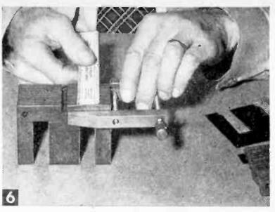
Clamp the stack of transformer laminations tightly together when you measure thickness. The thickness x the center leg width is the cross sectional area of core.
