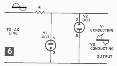
AC REGULATOR SCHEME EMPLOYING GASEOUS VR TUBES. R IS DETERMINED BY LOAD OUTPUT IS APPROXIMATELY 95 VOLTS
