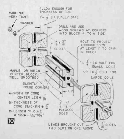
wire by taking a few turns around the bolt on the chuck side of the form. Set your counter at zero and wind back and forth as evenly as possible to avoid unnecessary wire crossings. When the counter reads 344, cut about a foot beyond the last turn, slip on spaghetti tubing, and bring the lead out through the same slot used at the start. Again, secure the lead with paper Scotch tape and a few turns taken around the bolt.
