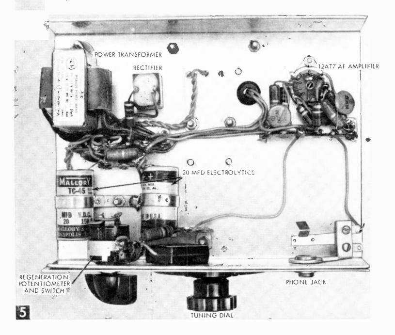
Now, wire the audio amplifier. Temporarily install the 'phone jack, and wire the output audio amplifier stage.
