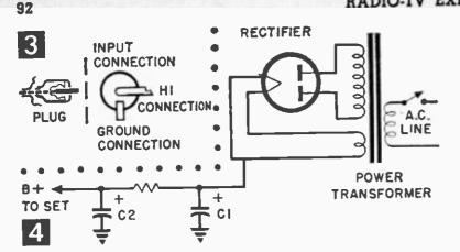
A broken shield or disconnection from plug ground or a faulty or open input jack can cause hum pickup.
