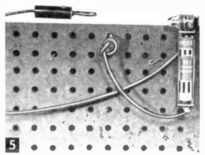
Short checker (indicator of right answers) mounts on the back of the board with bulb visible from front.
