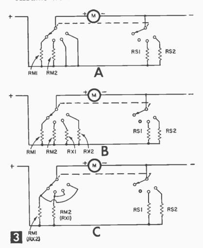
Means of switching various multipliers and shunts into meter circuits: (A) when only multipliers and shunts are used, (B) for extending the voltage rating by using special multipliers, and (C) for extending voltage by using the voltage multipliers themselves.
