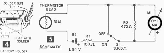
doesn't move, one of your leads is not perfectly soldered. Resolder, noting that the meter should deflect when a good joint is obtained. Blow lightly on the thermistor and the reading should change.
