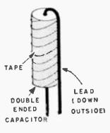
to extend the lead. Wrap the capacitor body with electrical tape to avoid any possibility of the bare wire lead accidentally shorting out to other adjacent components. This modification brings both leads out at one end, thus converting the component into a single-ended one, useable in printed circuits.—JOHN A. COMSTOCK.
