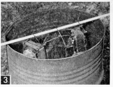
Burning a half hour will loosen the insulation and wrappings so that core laminations can easily be removed.
