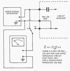
7 INPUT IMPEDANCE MEASURING CIRCUIT AND CALCULATIONS
