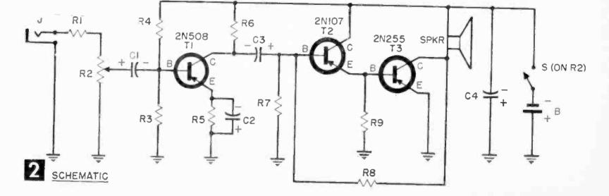
of the 2N255 from overloading the preamp. The driver output from the emitter of the 2N107 is directly coupled to the 2N255. R8 provides dc stabilization and a considerable amount of audio feedback.
