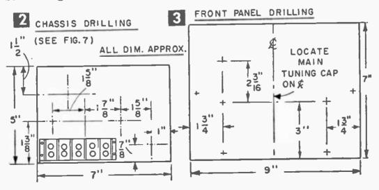
ing out the chassis as shown in Fig. 2. Set the tubes and coil in position in order to assure proper clearance, then drill all small holes with a No. 27 drill, large enough to clear the body of a 6-32 screw. Punch socket holes with a  $1\frac{3}{16}$ -in. Greenlee socket punch (available from any large radio supply house).
