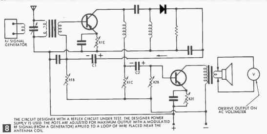
may be bypassed with electrolytic capacitors (about 10 mfd) for increased gain. The desired dc stabilization will be retained.
