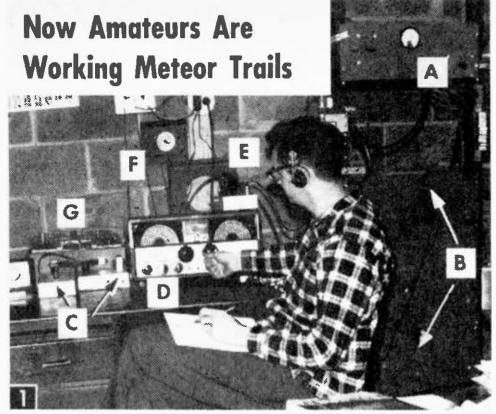
Here Walter Bain demonstrates the equipment needed to get into meteor trail work: A) transmitter; B) transmitter power supply; C) frequency marker; D) communications receiver; E) crystal controlled converter; F) clock with sweep second hand; G) tape recorder (optional).
