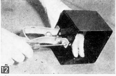
After fastening switch through its hole in handle with locknuts, attach handle frame to amplifier housing. Note that housing has been finished with primer, then black enamel lightly rubbed with steel wool.
