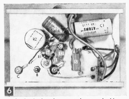
Under-chassis view shows parts layout and wiring.
