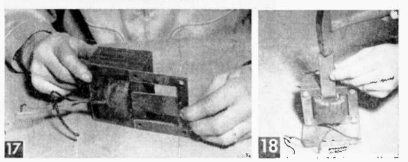
Left. Assemble the laminations alternating the E each layer. Usually longer E pieces cover the ends. Right, Fiber wedges driven into the open center spaces prevent vibration of the laminations.
