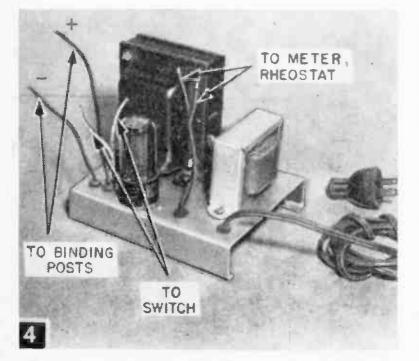
Top view of power supply shows components used. Wires through grommets lead to panel mountings.
