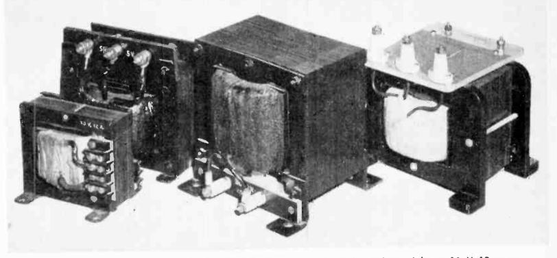
Transformers built using methods described in this two-part article. Left to right: a 10 V 12 amp filament transformer; a 10 V 25 amp filament transformer; a 3000 V 400 ma. plate transformer; a 2000 V 350 ma. transformer for large Tesla coil.
