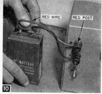
Difference of pin diameters insures right hookup for high voltage charge. As further safety measure, positive lead has red covering, matching color of positive terminal on panel.
