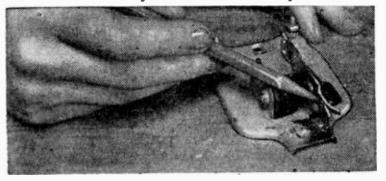
• This little relay will handle as much as two amps. without trouble. Remove stationary contact of an electric bell or buzzer and turn it around. When current flows through coil, armature is pulled in and it makes contact with stationary member.-R.F.Y.
