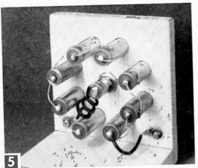
Flexible pigtail lead to end of switch assures reliable contact. A more rigid wire soldered to bearing might deliver unstable voltage due to corrosion between bearing and shaft.
