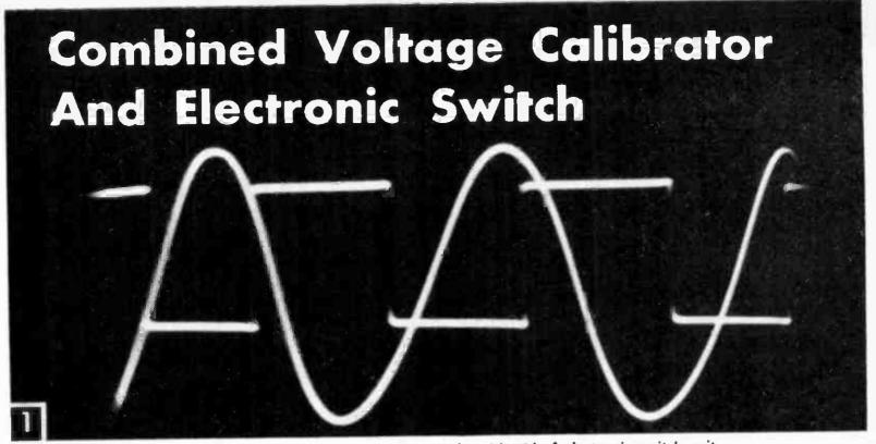
Sine and square wave seen simultaneously with aid of electronic switch unit.
