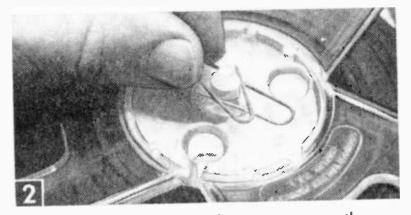
With the reels clipped in place, you can run the recorder tipped at various angles to pin down the source of rattles and vibrations.
