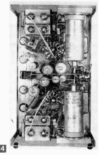
Back-of-panel view of the capacitor substitution box.
