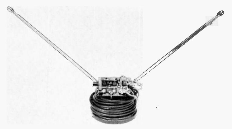
You can easily check the radiation of your station with this field-strength indicator.
