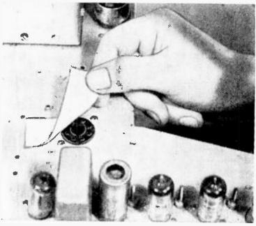
• When soldering on top side of radio or TV chassis, dropping solder in an open tube socket can cause trouble. Eliminate this possibility by placing a strip of wide adhesive tape over the open socket.—H. LEEPER.
