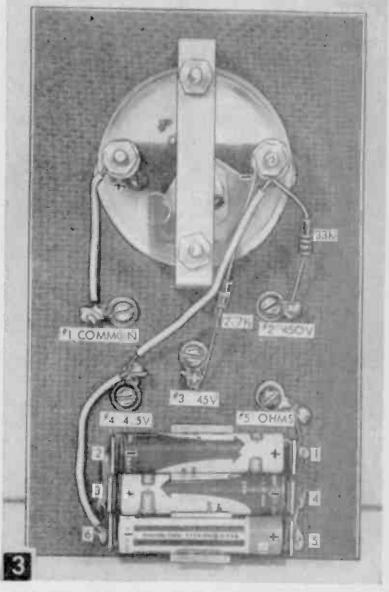
Parts mounting. Piece of #18 wire (arrow) supports battery holder.
