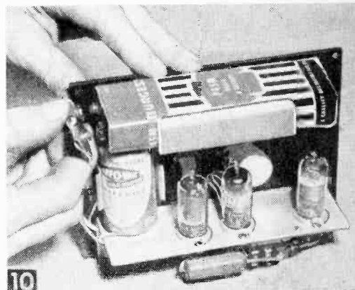
10 Tubes and batteries have been positioned and the snap-on terminals at the B battery are being pressed on. A piece of adhesive tape should be placed between the lower terminal of the A battery and the chassis so that this terminal will not short to the chassis. Note the tone control located between the two widest spaced tubes. Be sure that the 3V4 tube is next to the A battery or is in the output jack circuit.
