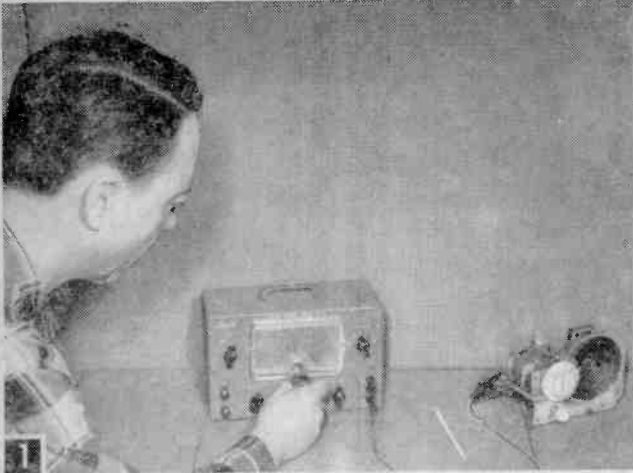
Signal Generator output cable connects to radio antenna and ground. A plastic blade screwdriver is only tool needed.
