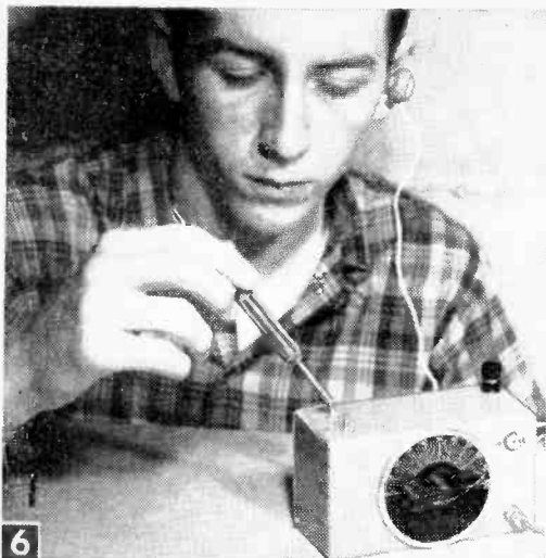
6 Coil slug screws extend above cabinet allowing for easy alignment. Here tuner is used with miniature earphone as a personal set.
