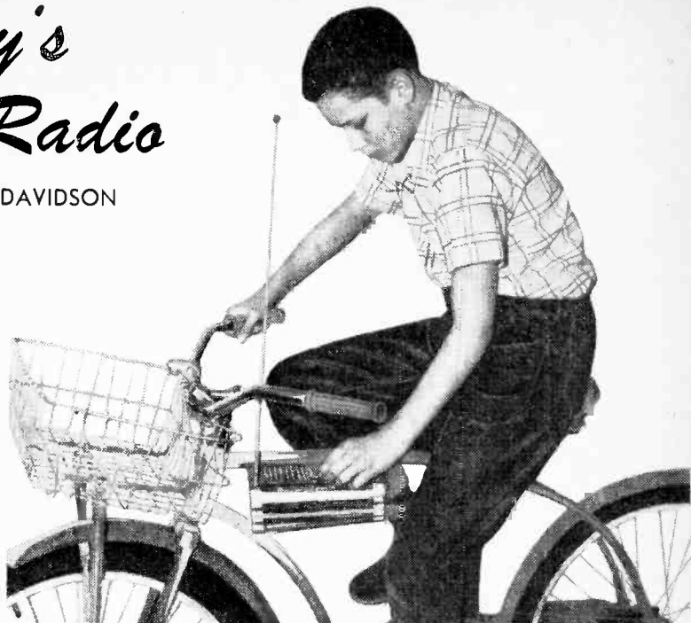
Have radio, will travel with this compact superhet receiver. Stripes were painted on plastic case by masking with tape and using paint from spray cans obtainable at hardware and 5- and 10-cent stores.
