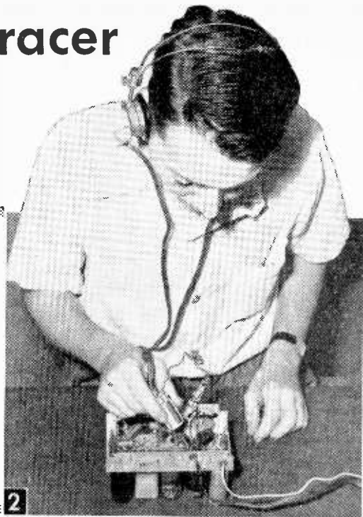
Tracking down the trouble in a radio set by following the signal through the grid and plate of each tube socket. Signal tracer built in a 1x2 in. plastic salt shaker. Alligator clip attaches to the ground or B- circuit of set being checked.
