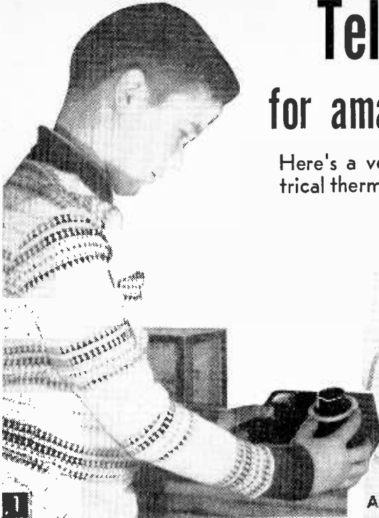
Telethermoscope indicator located inside house gives accurate reading of outdoor temperature. Three-wire cable shown in insert A connects temperature-sensing bulb, which is located outside, to box housing indicator meters.
