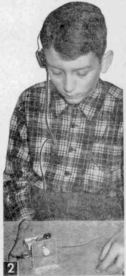
This midget super-regenerative set has pulled in stations 1500 miles away with good volume. For headphones, use a single or double type of not less than 2000 ohms.
