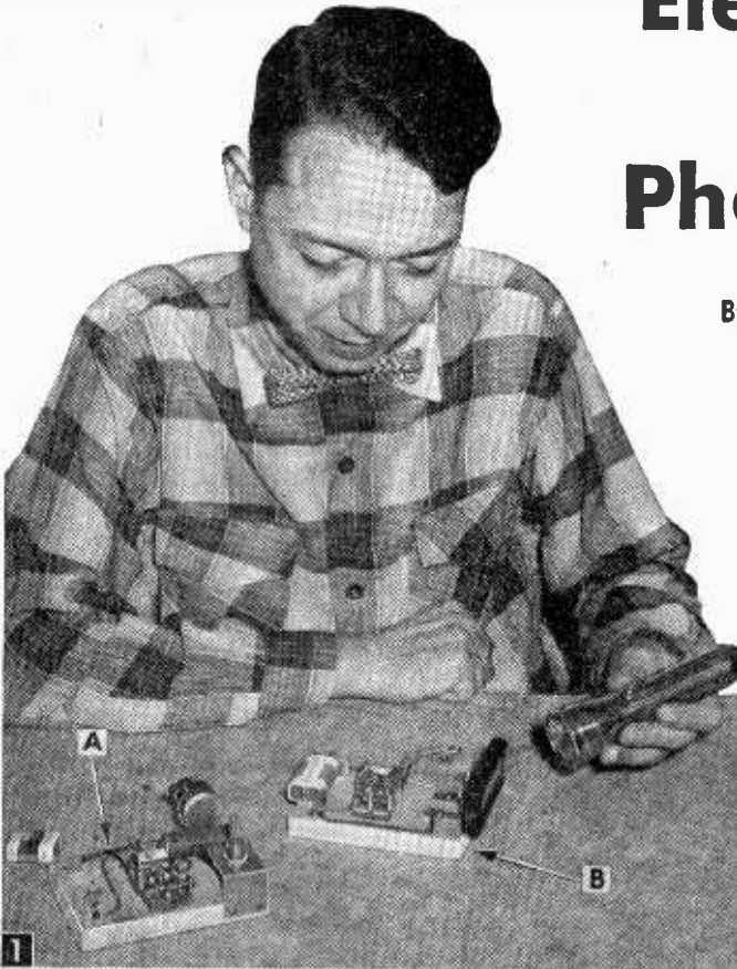
Fractional timer (A) and photoelectric eye (B) which use transistors require a minimum of parts and a single battery voltage source unlike identical but more complex vacuum tube devices.
