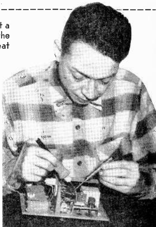
Wire solder is best handled by cutting three ft. off the spool, winding it on a pencil, and fishing one end through the spiral. As it is consumed, more is pulled through.
