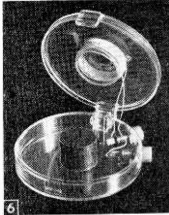
6 Under-the-pillow speaker built from a plastic stickpin case. Coil is wound on a plastic tube, and connecting cord plugs into the phone-tip-jacks.
