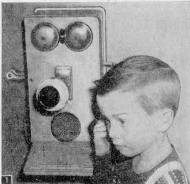
Rural crank-type telephone houses radio. Youngster is listening to other member of family through intercom hook-up of old telephone.
