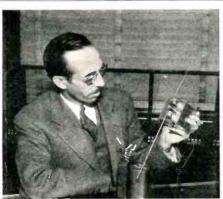
O. B. Hanson, Chief Engineer at the National Broadcasting Company, with the world's smallest Micro-wave transmitter, capable of flinging the humon voice a distance of four miles. It operates on wave-lengths of one meter or less at a power of .2-watt and was developed under Mr. Hanson's direction.
