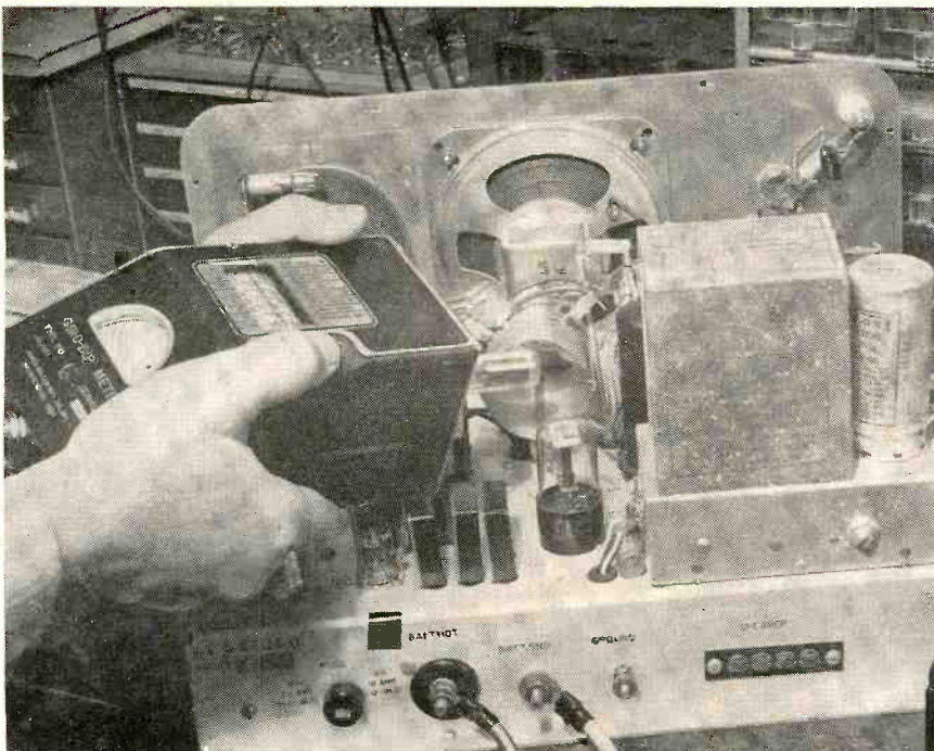
▶ Transmitter circuits can be pre-resonated with a grid-dip meter.
