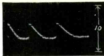
▶ (Left) Defective condenser across cathode resistor of horizontal output stage gave this wave form at the cathode. (Right) Wave form with condenser replaced.
