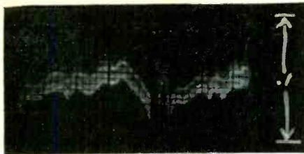
▶ (Left) Scope pattern at agc line when defective filter capacitor was in circuit. (Right) Photo of the pattern at the same point when the capacitor was replaced.
