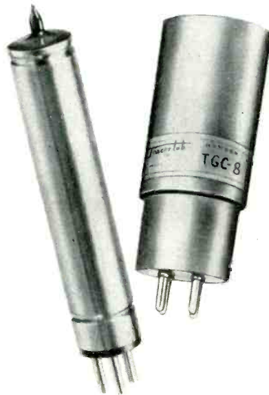
Fig. 1—Two typical Geiger-Mueller tubes. The one on the left is the Type 75NB3 manufactured by Amperex Electronic Corp. The one on the right is a Tracerlab TCG-8.
