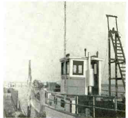
The typical marine end-fed Marconi antenna. Its rugged construction is a prerequisite for all-weather operation. Note that the mast is swivel-mounted, an expedient which allows it to be lowered while passing under low-clearance bridges.
