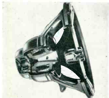
Fig. 1A—Photo shows cutaway view of Jensen Hi-Fidelity Triaxial three way loudspeaker. Letters "A" and "B" indicate the horns which couple the high range and middle range metal diaphragms to the air load. Refer to Fig. 1B for drawing of this speaker.
