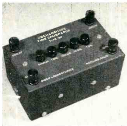
Fig. 4. Time Calibrator; Owen Model 160.
