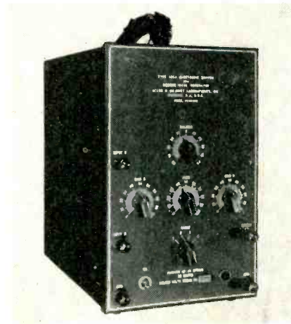
Fig. 7. Commercial electronic switch.
