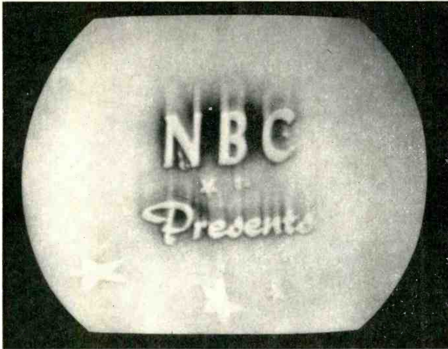
Fig. 4. Typical picture that may result because of vertical jitter.
