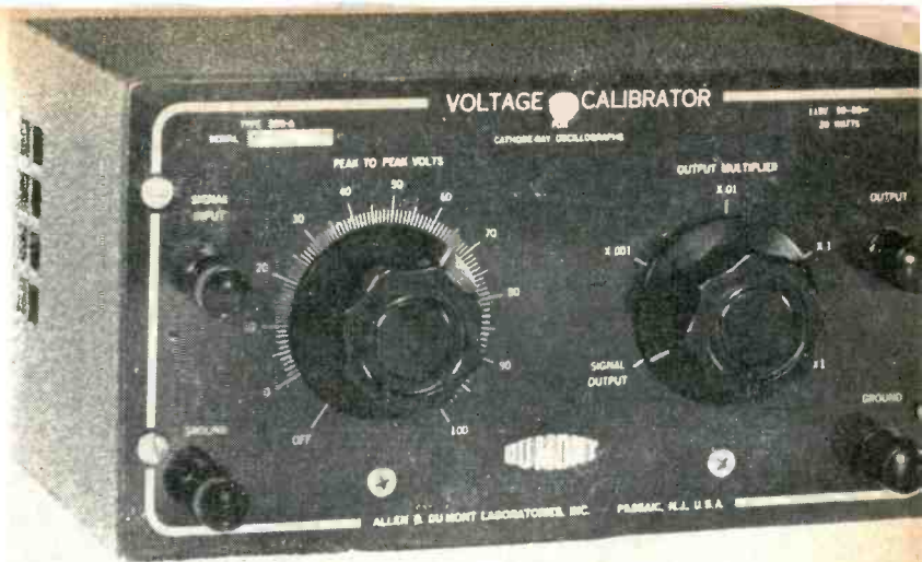
Fig. 2. The DuMont Type 264 Voltage Calibrator.
