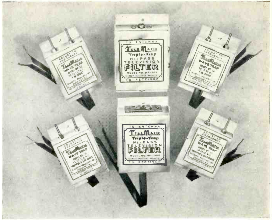
Fig. 10. Various types of TVI filters and wave traps which form a convenient kit for use by the serviceman in tracking down and eliminating TVI.
