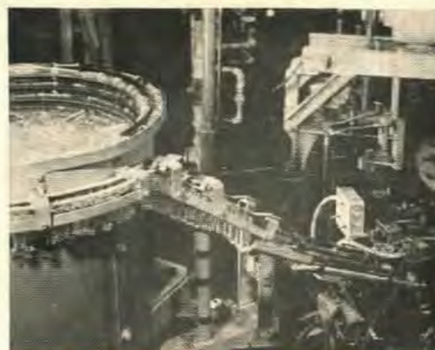
Cylindrical machine at left gently vibrates glass tube envelopes, urges them to climb inside track and automatically feed down ramp to tubulating machine. Tubulating machine etches tube type on envelopes, cuts glass to precise tube size, attaches exhaust tube to envelope to allow creation of a perfect vacuum.
