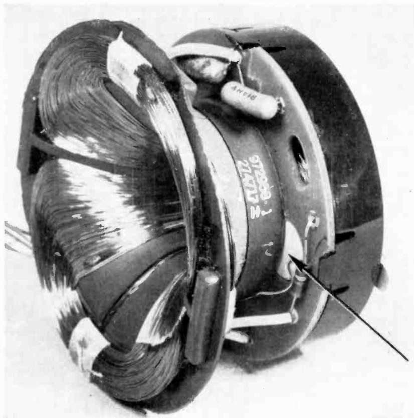
Fig. 1—Typical 110° deflection yoke. The arrow points to a thermistor, R133. Note magnets used to minimize pincushioning.
