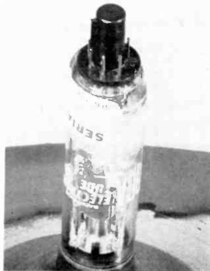
Fig. 3—Base of 110° kinescope showing straight thru pins and indexing plug.
