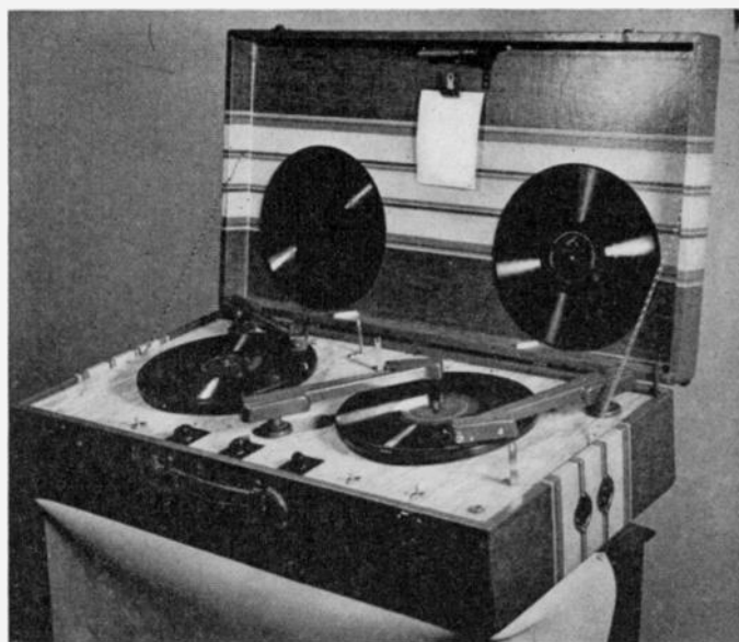
View of the dual-turnstile, triple-pickup record player for movie work or continuous musical reproduction.
