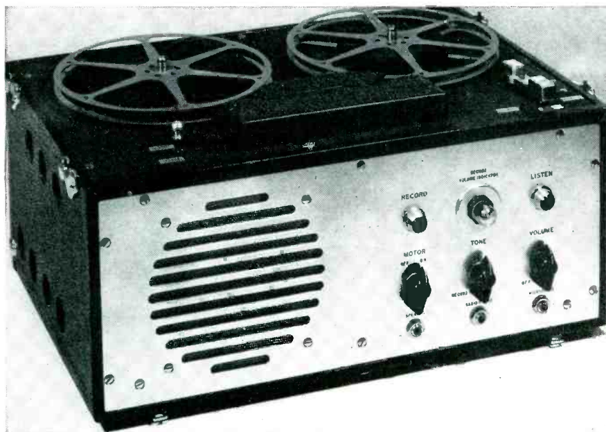
Front view of the magnetic tape recorder machine developed by Indiana Steel Products Company. Reels contain magnetized paper tape.
