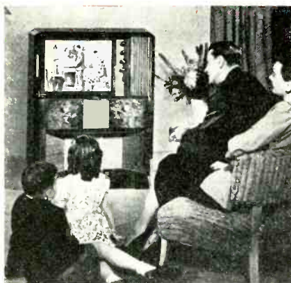
Large screen television receiver RCA-Victor Model 648 PTK: image size of newspaper page. Image is received on the face of brilliant 5-inch tube pointing downward; this is reflected by a dish-shaped mirror near base of receiver through a correcting lens to a mirror set at 45-deg. angle at top of set which reflects the picture through the back of special-type translucent screen. Set comes with AM, FM and shortwave radio reception, with pushbutton tuning.
