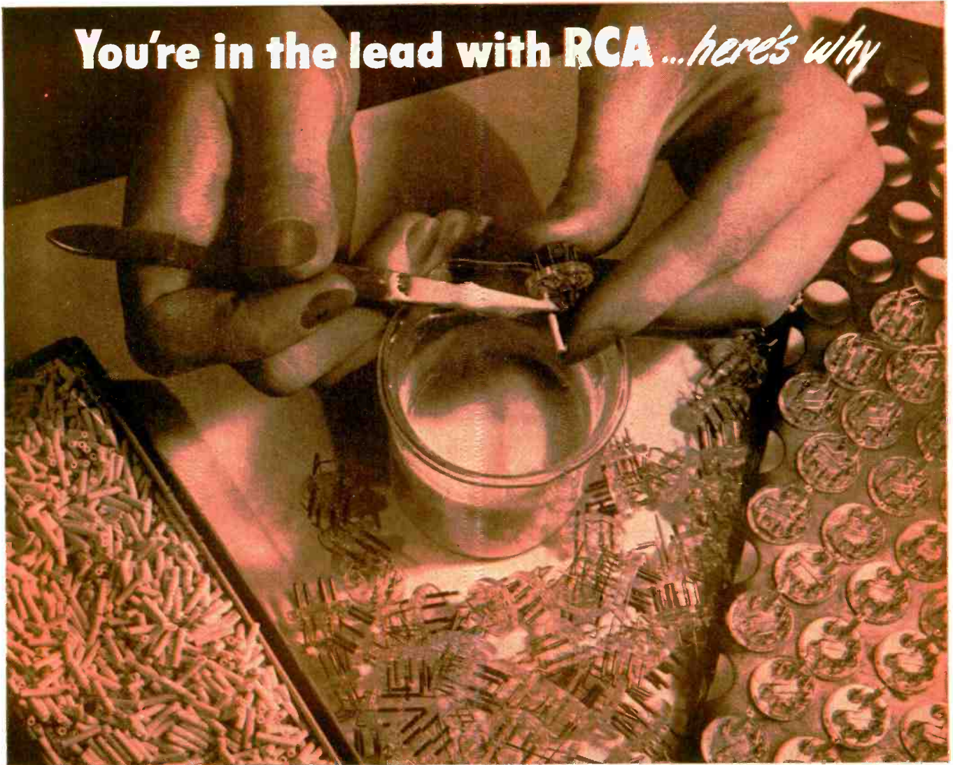
Cementing ceramic insulator to miniature tube button stem — one of the many delicate operations in making an RCA tube that calls for unusual skill.
