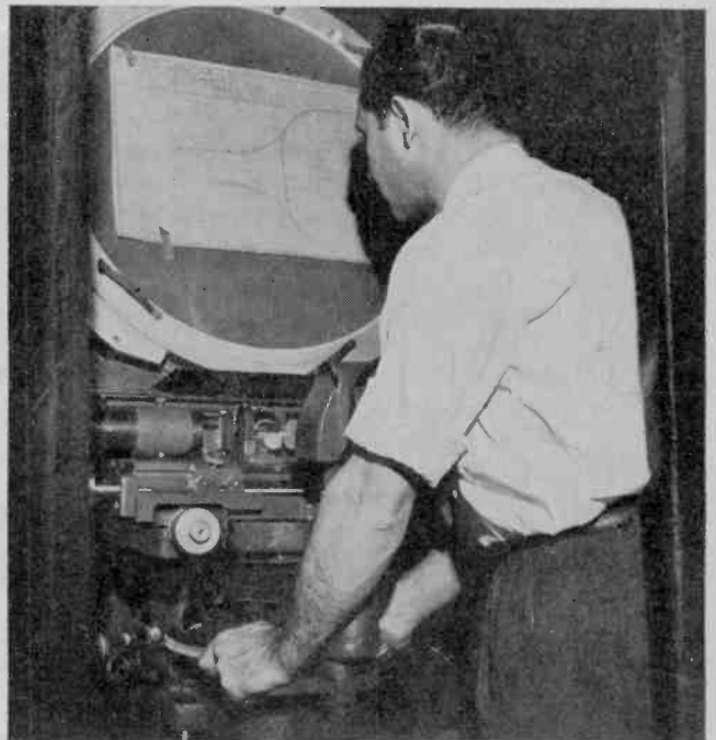
Tiny tube parts are magnified and their outlines superimposed on scale drawings to insure meeting the extremely close dimensional tolerances required.
