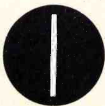
Fig. 4. Indication Caused by AC Voltage on Vertical Plates With No Sweep
