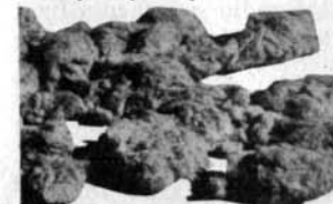
Cotton filler, used in inferior covers, bunches up in corners leaving bare spots—dangerous for fine surfaces.
