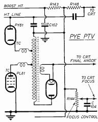
From the circuit diagram it will be seen that the short from the junction of R143/R148 was in effect cleared when the focus control centre tap was turned to the earthy end of the track. Replacing the 0·1µF capacitor restored the circuit to its proper working conditions.—D.Mc.L., Lochgilphead (1050)
