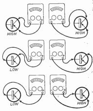
Fig. 2: Typical measurement of transistor with  $20,000\Omega/V$  meter. Note that the positive terminal refers to polarity at meter (ohm-meter battery may apply positive voltage to negative terminal of meter). Do not take these readings with transistor Incircuit. Use Ohms X100 range of meter.
