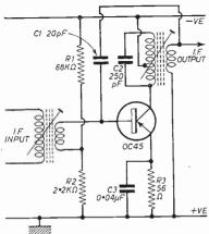
Fig. I: Typical[transistor i.f. stage.
