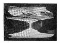
The trouble, however, in spite of its formidable symptoms, turned out to be nothing more involved than a heater-to-grid leak (of 500kΩ) on the PL81 line output valve.—F.C., Crewe (1076).
