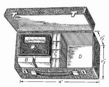
It is in four sections, as shown in the drawing. The leather partitions are about an inch shallower than the base, allowing one to overlay the compartments with a soldering iron, valve manual and duster. The iron shank and bit are housed in a tubular spanner ½ in.× ½, standard size for potentiometer locknuts.
