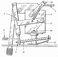
Fig. 2: Side view of the switch mechanism used in the Motek KIO tape deck.
