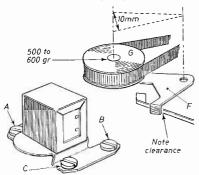
Fig. 4: (Top right) Tension wheel mounting in Philips tape decks.
