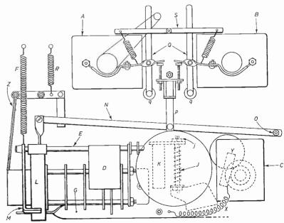
Fig. 1: Underside view of the Motek K10 tape deck showing the main components of the mechanism. (This drawing is not to scale)
