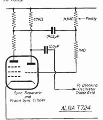
The  $47k\Omega$  anode resistor was correct. as was the 0.02 µF coupler from the anode of the sync separator (pentode section). All that was left was the fixed potentiometer in the grid circuit, which consists of a  $3.3 M\Omega$  and a  $1 M\Omega$  in series from the h.t. line, with the  $0.02 \mu F$  coupler taken to their
