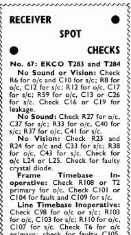
Cl07 for s/c. Check T6 for o/c. primary; check for faulty Cl05, Cl06, Cl11; check L32 for leakage to the core. **No Raster:** Check C93 e.h.t.
