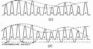
The filtered complex wave fed to the frequency modulator has a frequency spectrum consisting of A+B at audio frequency, A-B DSB a.m. on a suppressed subcarrier at the sampling frequency, and A+B DSB a.m. on a subcarrier at the second harmonic of the sampling frequency (see Fig. 3). Audio bandwidth is usually 15 kc/s and the sampling
