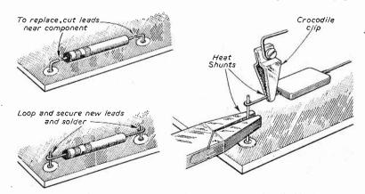
Fig. 2: Details of removing and reconnecting components, as described in the text. APRIL, 1960
