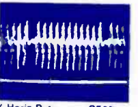
1/2 Horiz Rate 1.25 VPP Q501 Collector
