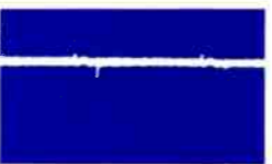
19. EMITTER, B-Y DEMODULATOR (Q20), 0.7V P-P, HORIZ. EMITTER, R-Y DEMODULATOR (Q21), 0.9V P-P, HORIZ. (PWS1)
