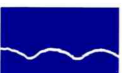
11. RIPPLE of CH 10C, 0.1V P-P, VERT. UNDERSIDE CHASSIS NEAR TH73 (ON SCHEMATIC)
