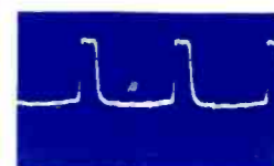
32. CATHODE, BURST GATE DIODE, (CR19) 12.5V P-P, HORIZ. (PWS1)
