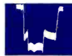
4 1.9V P/P, 15.750Hz Hor. Sync. Pulse Showing 4.5MHz Trap out of Adj.
