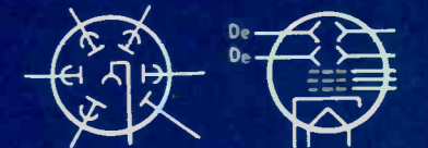
Photomultiplier Tube Cathode-ray Tube with Electrostatic Deflection. Remove De for Magnetic Deflection
