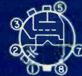
UHF triode (disk-seal type) with internal capacitor. Tube terminals added as shown where desired
