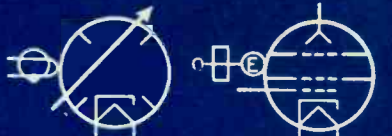
Magnetron Tunable, Loop Coupled Reflex Klystron Integral Cavity, Aperture Coupled
