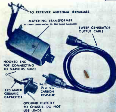
Fig. 3 IF-RF Alignment Fixtures
