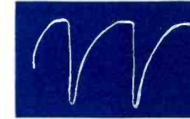
Fig. 17. Horizontal Oscillator, 43 volts, 15,750 c.p.s. test point.
