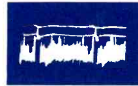
Fig. 11. Sync Separator Grid, Pin 7, 38 volts, 60 c.p.s.
