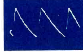
Fig. 16. Phase Comparator, Pin 6, 7 volts, 15,750 c.p.s.
