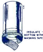
Figure 19. Special Tube Shield for IF Alignment and IF Response Curve Check.
