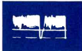
Fig. 9. Composite Signal, Pin 2 of 12BY7, 6 volts, 15,750 c.p.s.
