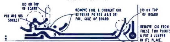
View of Wiring Side of Printed Board.
