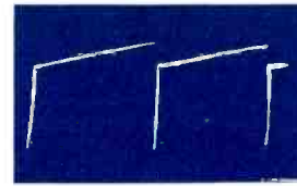
Fig. 14. Vertical-Output Grid, Pin 6, 80 volts, 60 c.p.s.
