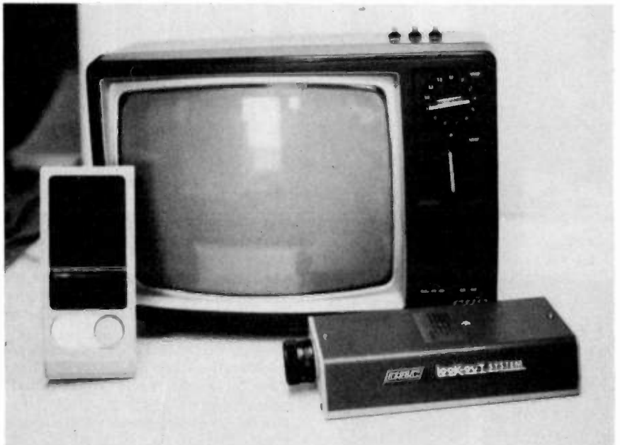
Fig. 1. The GBC Look-Out 2000 system, camera, monitor, and intercom speaker.
