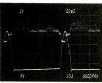
Fig. 9. Dual-trace scope indicates correct timing of the horizontal keying pulse.
