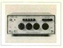
vernier to provide total dynamic range of 90dB. Precise frequency selection is possible with the 3 digit tuning selector. Simultaneous inverted (180°) and quadrature (90°) outputs also are provided. Each output is 7V RMS with 600 ohm source impedance. When combined with a distortion analyzer, such as the Krohn-Hite 6800 series, it provides a complete distortion measurement system. The 4400 is priced at \$550: availability is 60 days.
