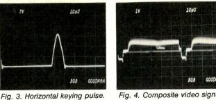
Fig. 4. Composite video signal.
