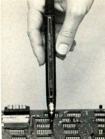
Fig. 10. A current tracer probe (courtesy of Hewlett-Packard).
