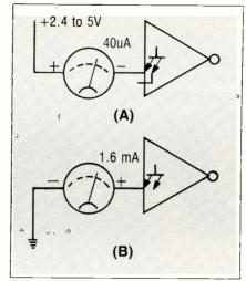
Fig. 12. Currents in TTL input circuits.
