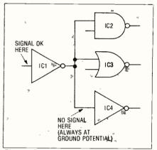
Fig. 14. Problems in isolating a short circuit.
