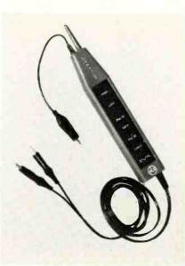
Fig. 6. A logic probe by Non-Linear Systems.
