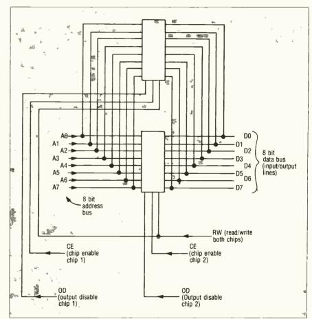
Fig. 1. A logic block diagram of a 512  $\times$  8 RAM organized with two 256  $\times$  8 RAMs. The "output disable" on each chip controls the tristate logic output of that chip. The "chip enable" input enables, or disables, the chip, and is used for chip selection. The "read/write" pin input determines whether we are reading, or writing, data.
