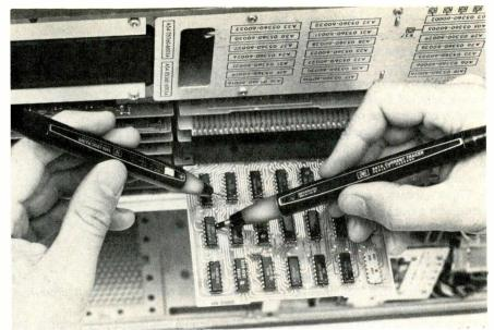
Fig. 11. Using a current tracer with a logic pulser (courtesy of Hewlett-Packard).
