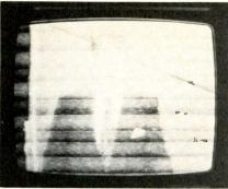
Fig. 8. Streaks caused by open filter capacitor at +24 volt input at pin W13.
