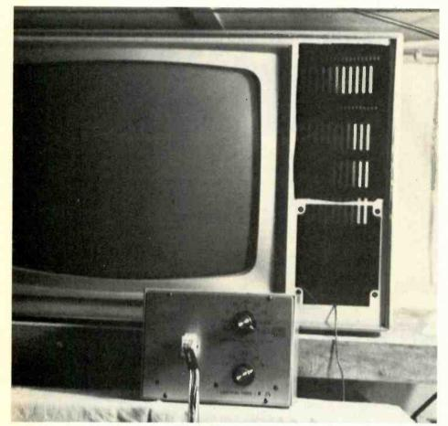
sis test jig or a junked TV set simply remove the original yoke and replace it with the yoke supplied with the 10J107. Reinstall the original convergence assembly and blue lateral assembly and use them for static convergence of the jig. Without a dynamic convergence capability, some edge misconvergence is normal with all test jigs.
