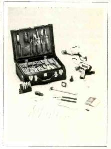
desoldering equipment, solderless terminals, % inch electric drill and more. In addition there is a selection of specialty and hard-to-find tools to reportedly handle almost any repair or service situation.
