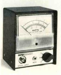
as a demodulator of AM transmission envelopes. The demodulated (audio) signal is available at a front-panel miniature phone jack to feed into high impedance display or analysis instrumentation. VSWR of model 6257 is below 1.1 to 512 MHz and less than 1.15 to 1000MHz in 50 ohm coaxial systems. The price is \$265.
