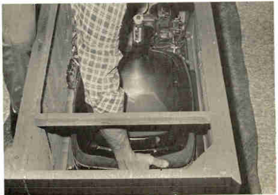
A5— The 25A tube is mounted through the rear of the cabinet.
