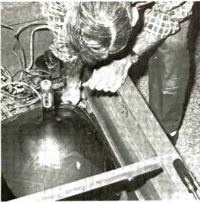
A6—The electronic technician manually adjusts all four mounting lugs on the band and lines them up with the mounting brackets.
