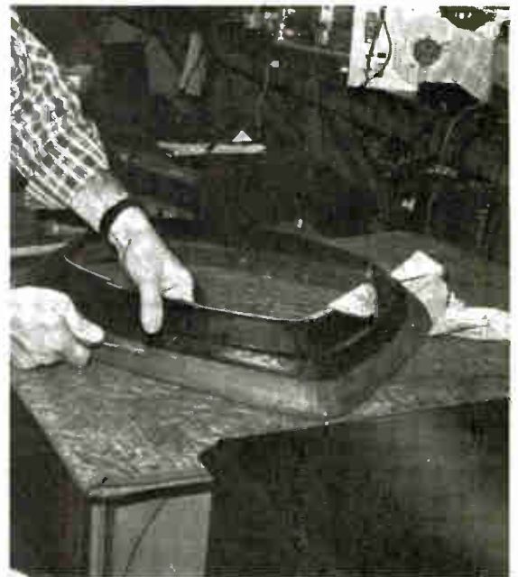
EG2—The beam shield is then cut and fitted over the 25EG. It goes on easily with spring-mounted loops. (The "Speed Fit" replacement for Zenith tubes includes a preassembled beam shield, a de-gaussing coil and adhesion pads already placed in position for the yoke.)
