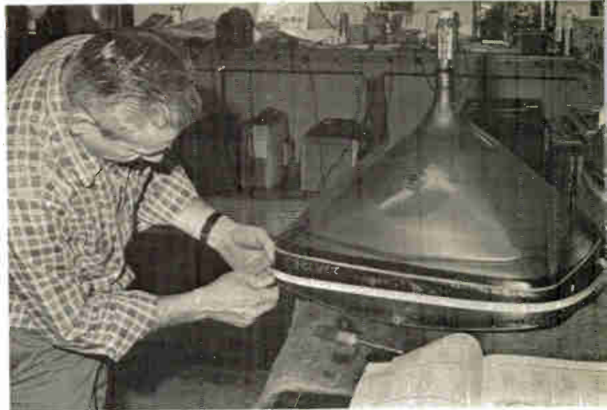
A3— The mounting band and four brackets are placed on the 25A tube.
