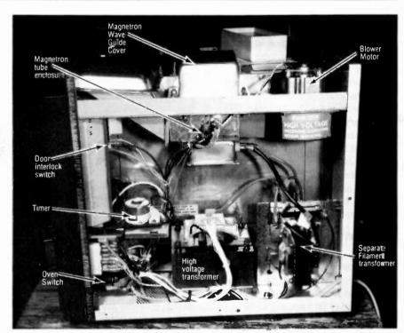
Fig. 1 The back metal cover is removed from the microwave oven showing the cooking mechanism.
