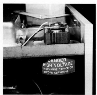
Fig. 5 Always discharge the high voltage capacitor before servicing a microwave oven. Many manufacturers place a very convenient sign to remind of this operation.
