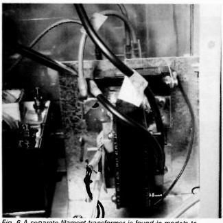
Fig. 6 A separate filament transformer is found in models to supply filament voltage to the magnetron tube. Notice the large high voltage transformer to the left.
