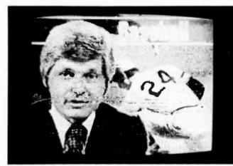
Fig. 1-Electrical arcing interference
