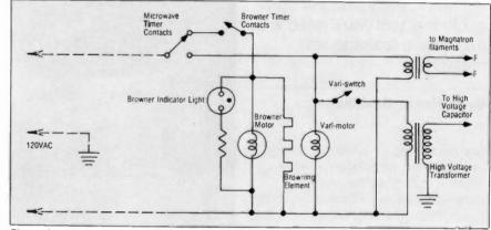
Fig. 4 A partial schematic of the browner unit.
