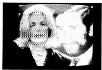
Fig. 4-AM (i.e. CB) interference
