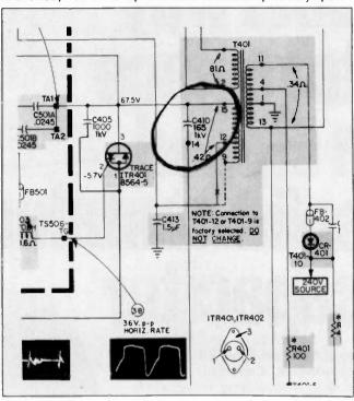
Color TV Chassis CTC72—No color except for a one inch multicolored vertical bar at the extreme left edge of the screen. The probable cause is a shorted CR306 diode.
