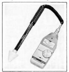
wave ovens, heaters, and dryers. It reportedly meets HEW performance standards and is suitable for service and repair use, as well as production testing. It is a hand held wide-range tester with four ranges of to  $100 \text{mW/cm}^2$  with accuracy of  $\pm$  1dB and a 1.2 second response time, according to specifications. The probe is priced at \$246.75, complete with batteries and manual.
