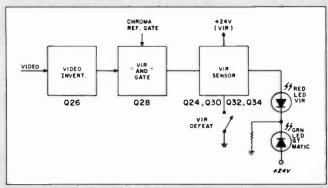
Fig. 5-Simplified schematic VIR sensor.
