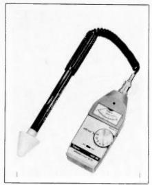
Fig. 2 Simpson's 380M microwave leakage tester.
