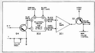
Fig. 7-Simplified schematic color control.
