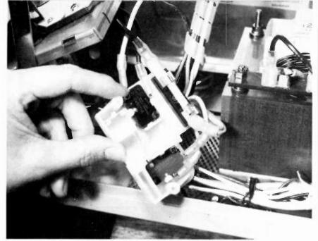
Fig. 8 Many microwave oven repair problems are caused by interlock switches. Either the switch goes bad or may need adjustment.
