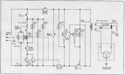
Fig. 3 A typical microwave oven schematic diagram. (Courtesy-Sharp Mfg. Co.)
