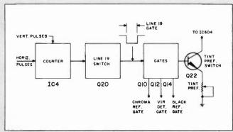
Fig. 4-Simplified schematic line 19 identifier.
