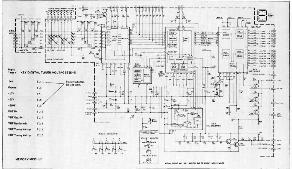
Fig. 2–The E49 digital tuner control. (Courtesy of GTE Sylvania)
