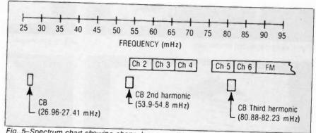
Fig. 5-Spectrum chart showing channels susceptible to interference
