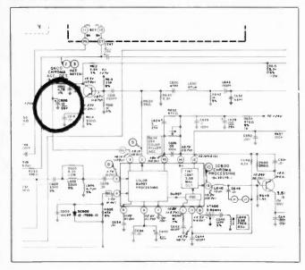
Color Chassis E21—No Vertical Sweep. Sweep drives normally with sweep analyzer. The cause was found to be a leaky C328 in the vertical linearity control circuit.
