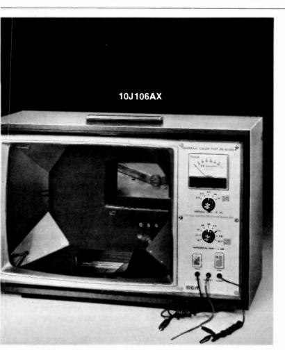
With the new RCA 10J106A Color TV Test Jig you can troubleshoot a TV chassis without bringing the cabinet and picture tube into the shop. The 10J106A helps you isolate picture tube or chassis malfunctions quickly, and without disturbing your customer's picture-tube alignment.
