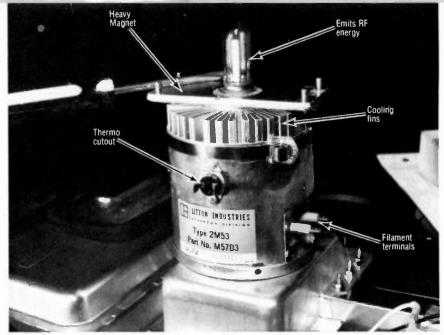
Fig. 7 Be very careful when working around the tube. The heavy tube magnet can pull tools from your hands.
