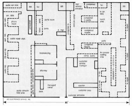
Fig . 3-Floor plan of Aid Electronics
