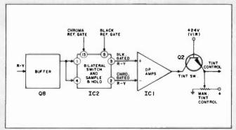
Fig. 6-Simplified schematic tint control.
