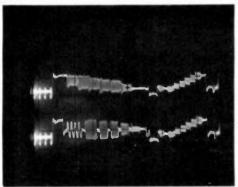
Fig. 2–Color bar and multiburst test signals displayed via delayed sweep at 10 usec/div with main sweep (showing lines 14, 15 and 16) at .2msec/div.
