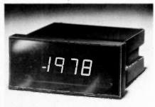
replace the popular Fairchild models 53, 75, and 78 3 1/2 digit units. The Model 78 case fits the same panel cutouts as the Fairchild, plus it has the additional feature of front mounting capability and panel locking retainers. It is available in 200mV, 2V, 20V and 200V ranges at 0.05% accuracy. Parallel BCD units are available as are 5v DC powered units. The Model 78 will be marketed at prices from 20% to 30% lower than Fairchild models in any quantity, offering improved design at low cost.
